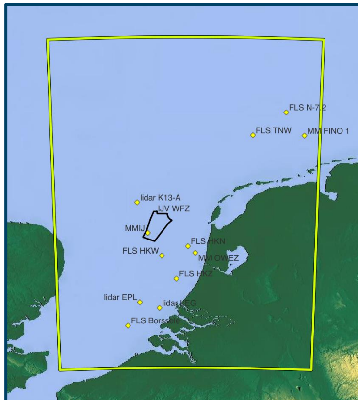
Figure 4.8 1.67 km Unified-WRF domain (yellow boundary) and measurement datasets used in the post-processing
