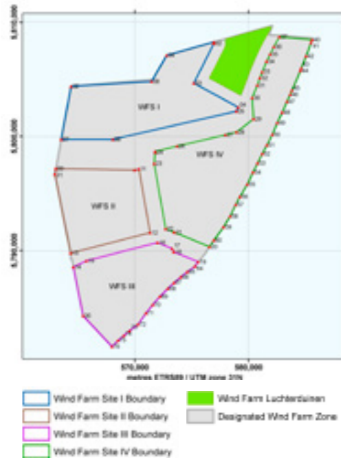
Figure 3c The Hollandse Kust (zuid) Wind Farm Zone and the corner coordinates of all Wind Farm Sites
