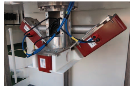
State of the Art Kongsberg Dual Head Dual Ping Multibeam in retractable moonpool system.
