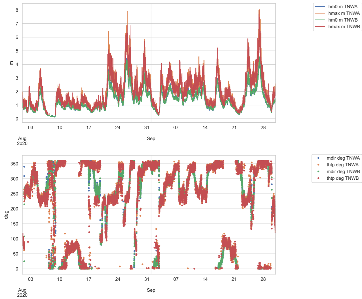
Figure 4.21 Wave height and direction from stations TNWA and TNWB during August and September 2020 correspond well.
