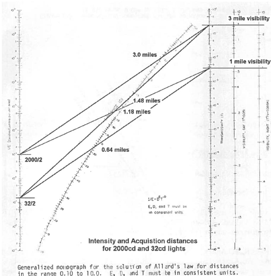
**Figure D-2 Intensity and acquisition distances of 2,000 cd and 32 cd lights**
