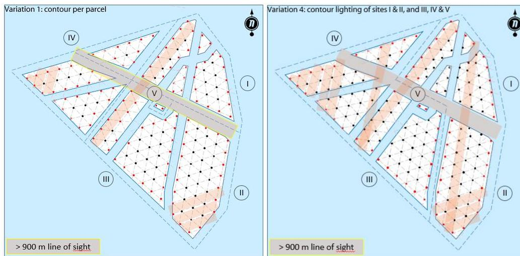
**Figure 16: Instances with >900 Meter line of sight with 1200 Meter grid and contour lighting for two variations**
