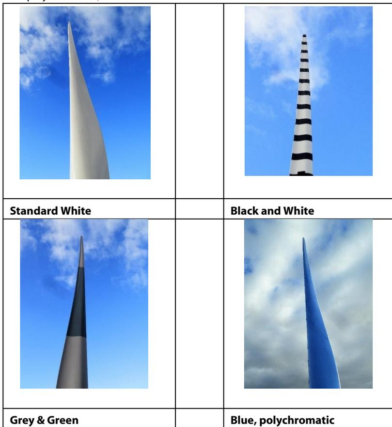
**Figure G-1 Wind turbine blades used for visibility testing**
