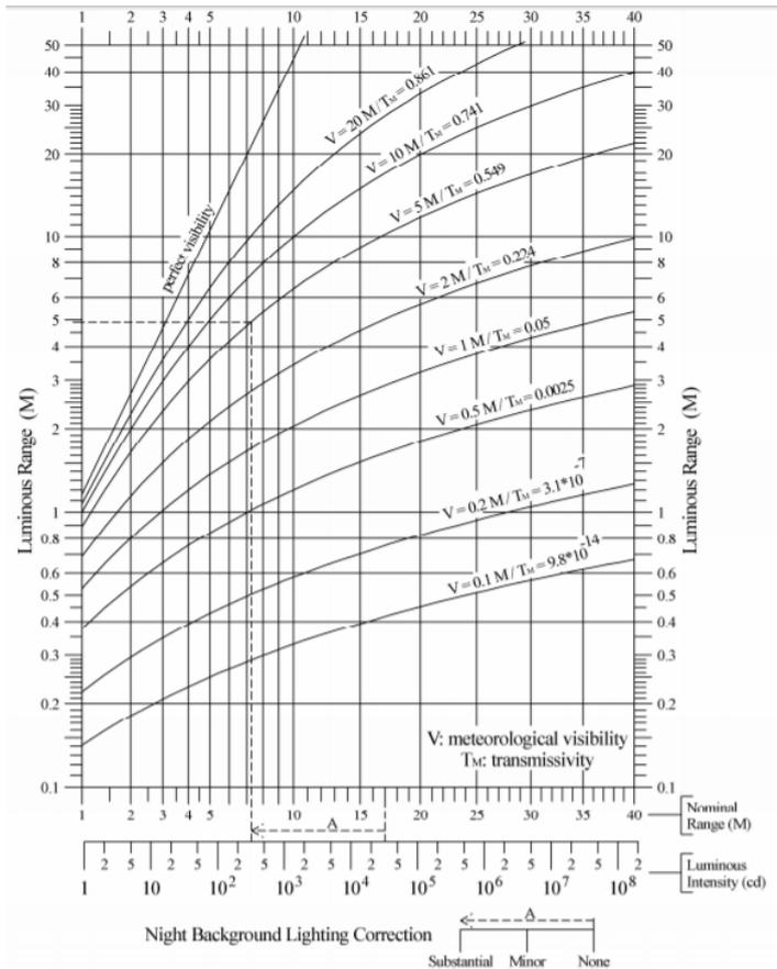
**Figure 17: Relationship between Luminous Intensity and Range (Source: IALA)**
