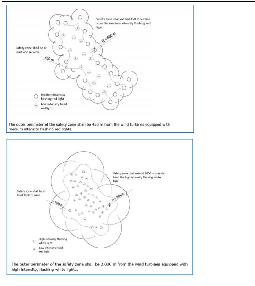
**Figure 4: Model of contour lighting from Finnish Transport Safety Agency**
