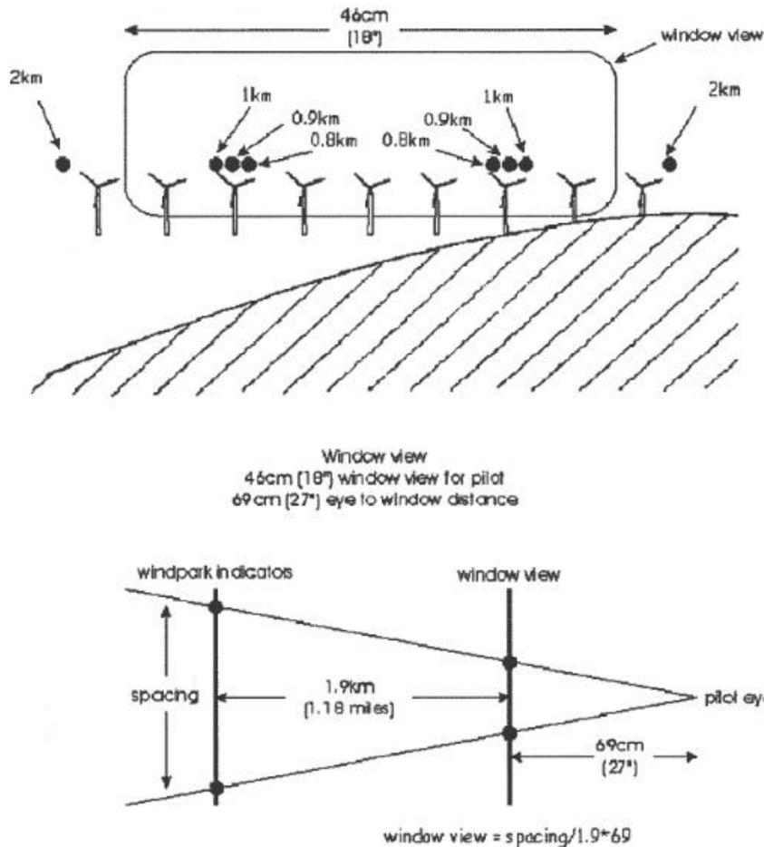
**Figure D-4 Visibility wind turbines**
