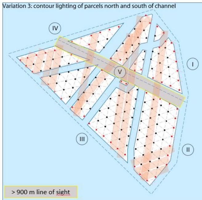
**Figure 13: Variation 3: Indicative layout of 1,200 Meter grid with contour lighting of parcels north and south of channel**
