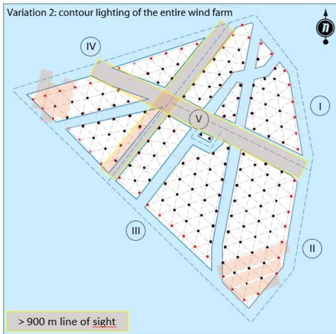
**Figure 12: Variation 2: Indicative layout of 1,200 Meter grid with contour lighting for entire wind farm**
