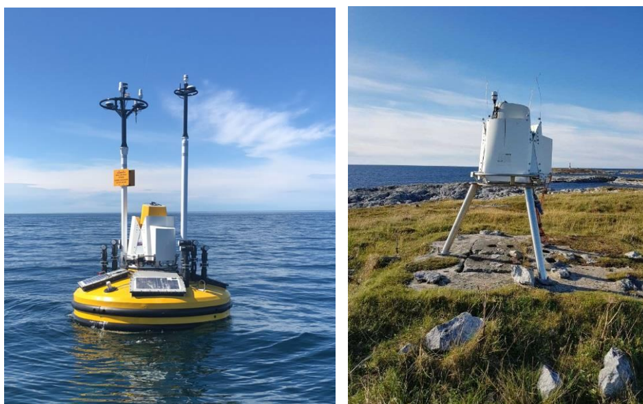
Figure 2: Seawatch Wind Lidar Buoy (left 1 ) and Reference Land Lidar as installed near/at Frøya test site.
