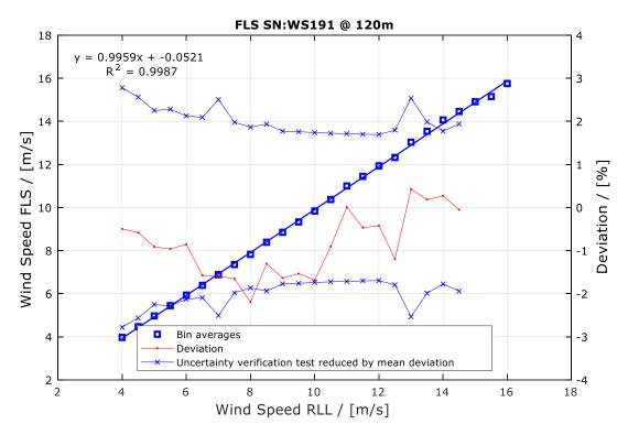
Figure 10: Bin-wise comparison of the horizontal wind speed component at 120 m
