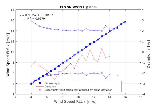
Figure 8: Bin-wise comparison of the horizontal wind speed component at 80 m
