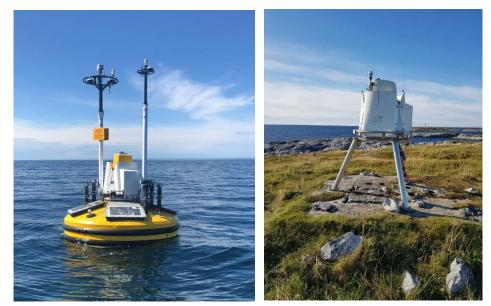
Figure 2: Seawatch Wind Lidar Buoy (left<sup>1</sup>) and Reference Land Lidar as installed near/at Frøya test site.
