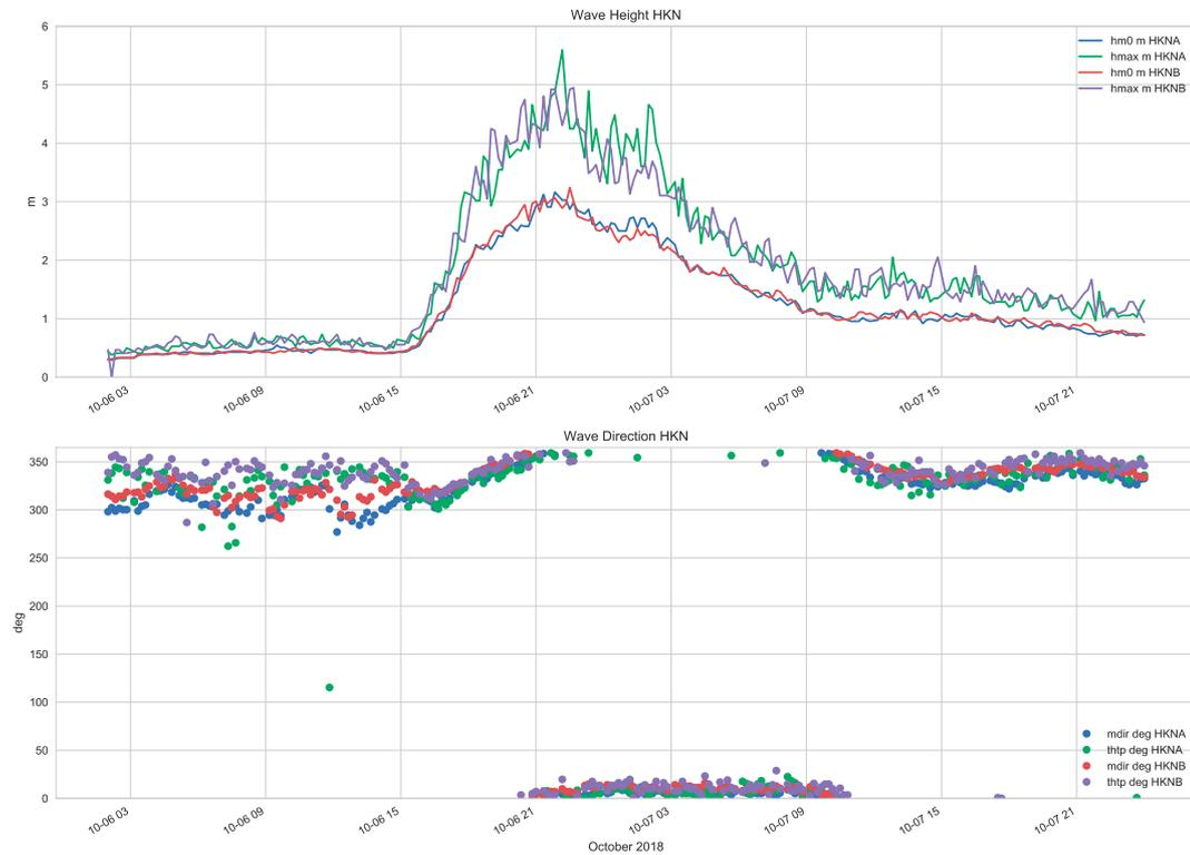
Figure 4u Wave height and direction from both buoys during the storm event in October 2018 correspond well.
