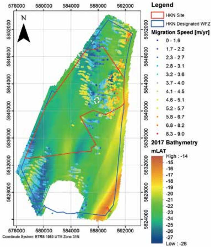
Figure 40 Map view of the measured bathymetry in 2017 and the mean estimated sand wave migration speed over the period 1996 – 2017; note that dots are only present at locations where sand waves are present.
