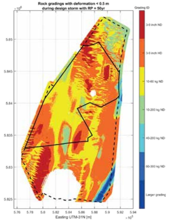
Figure 4r Spatial distribution of rock gradings that are expected to show less deformation than 0,5 m during the design storm with a return period of 50 years.
