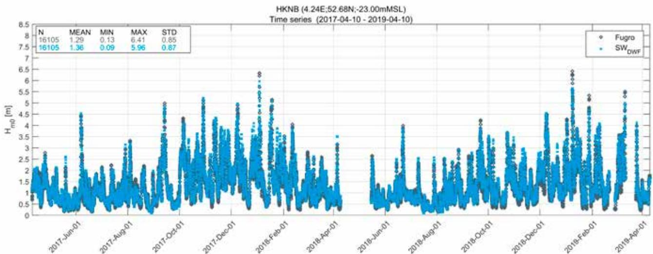
Figure 4x Time series comparison of significant wave height between model and measurements at location HKNB.
