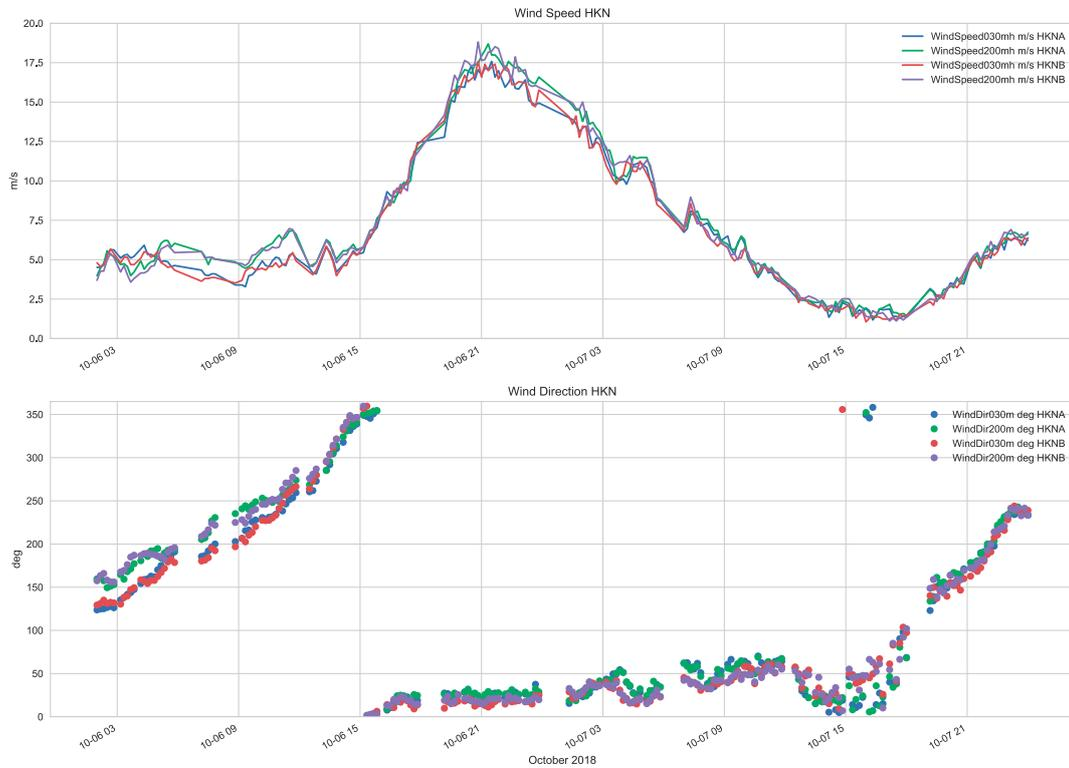
Figure 4t Wind speed and direction measured by the SWLB LiDAR at the highest and lowest heights for both buoys during a storm event in October 2018. The measurements correspond well.
