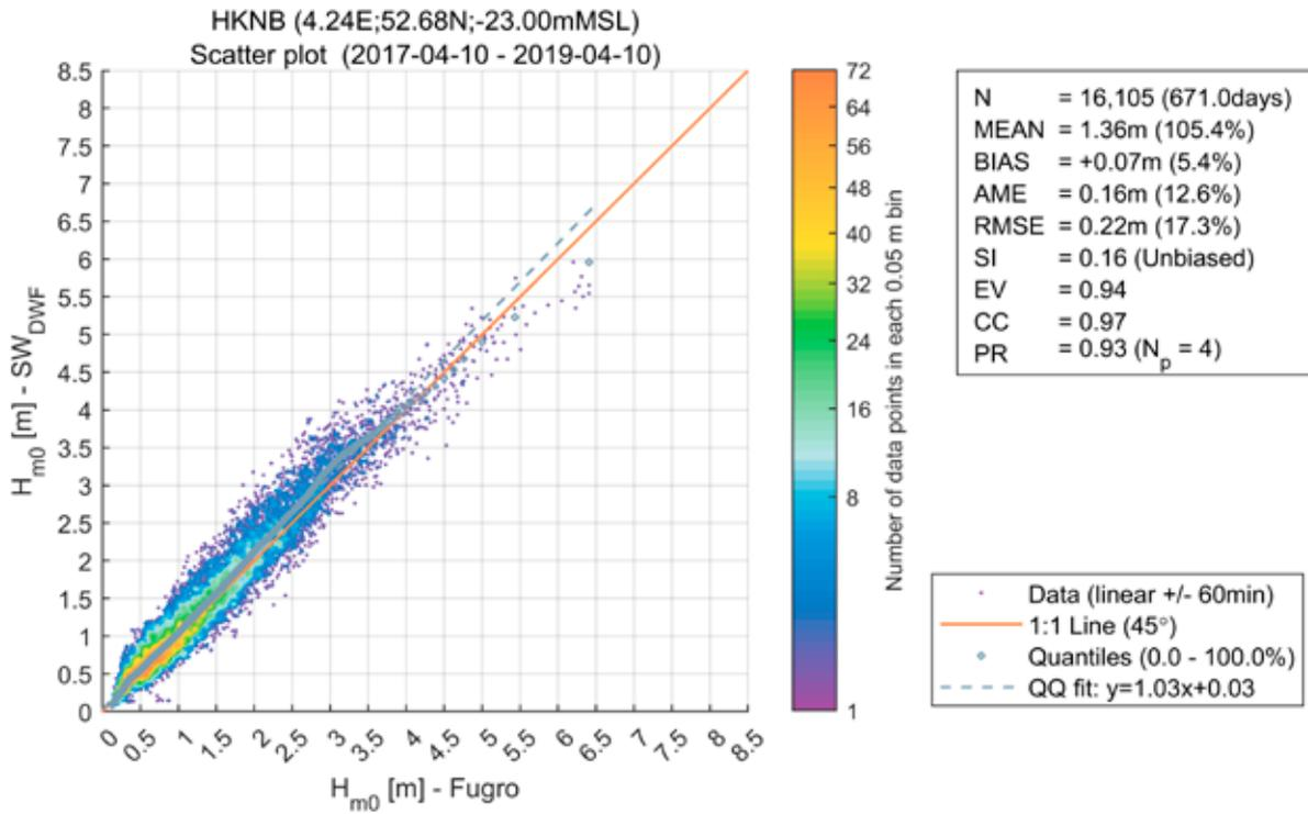
Figure 4w Scatter comparison plot of significant wave heights between the model and measurements at location HKNB.
