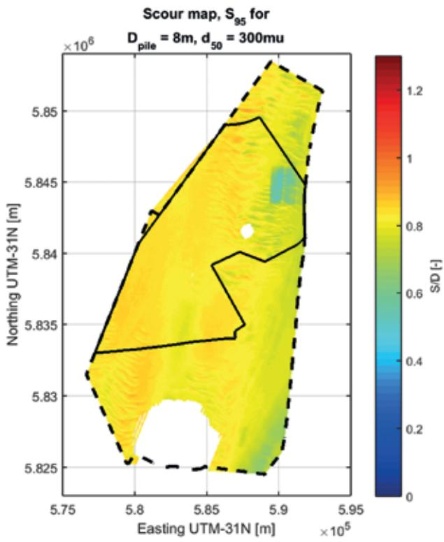
Figure 4q Map showing the 95%-non-exceedance value for the dynamic equilibrium scour depth ( $S_{95}/D_{pile}$ ) in the HKNWfZ, for one simulation with  $D_{pile} = 8\text{ m}$ ,  $d_{50} = 300\ \mu\text{m}$  and spatially varying hydrodynamics
