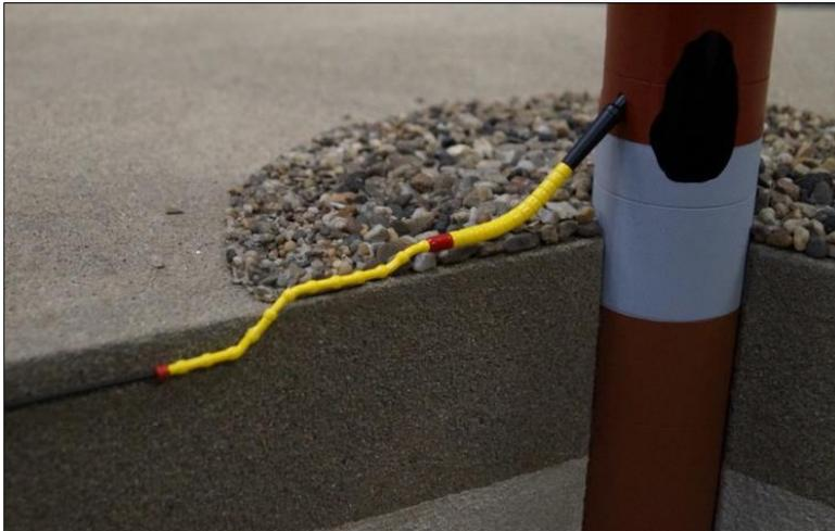
Figure 7-5 Monopile and anti-scour protection (OWF Gemini)
