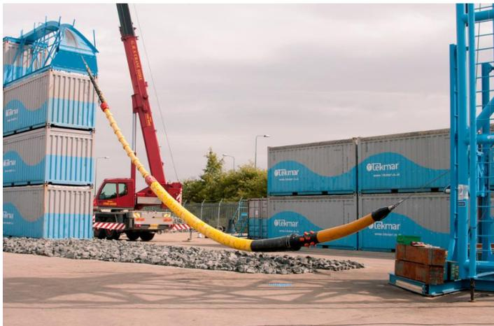
Figure 7-11 CPS under pull in testing (courtesy Tekmar)
