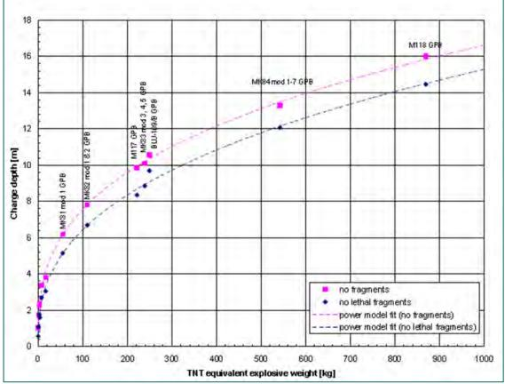
Figure 18: Minimal water depth to detain fragmentation of explosives with a Net Explosive Weight of 0-1,000 kg TNT equivalent [12].
