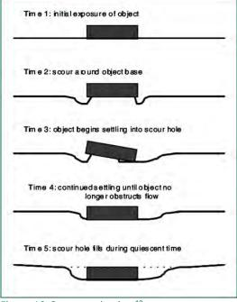
Figure 16: Scour mechanism<sup>10</sup>.
