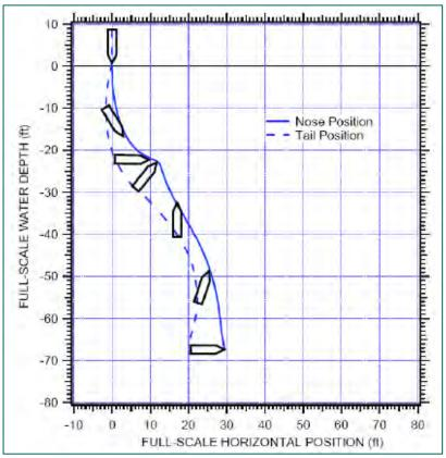
Figure 15: Trajectory of Mk 84 with no tail section and water-entry velocity of 296 m/s.
