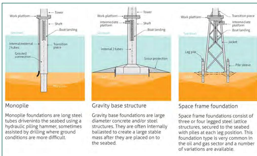
Figure 19: Example of suitable foundation types.<sup>24</sup>
