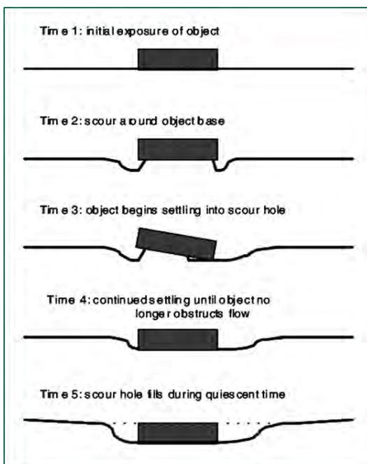
Figure 16: Scour mechanism<sup>10</sup>.
