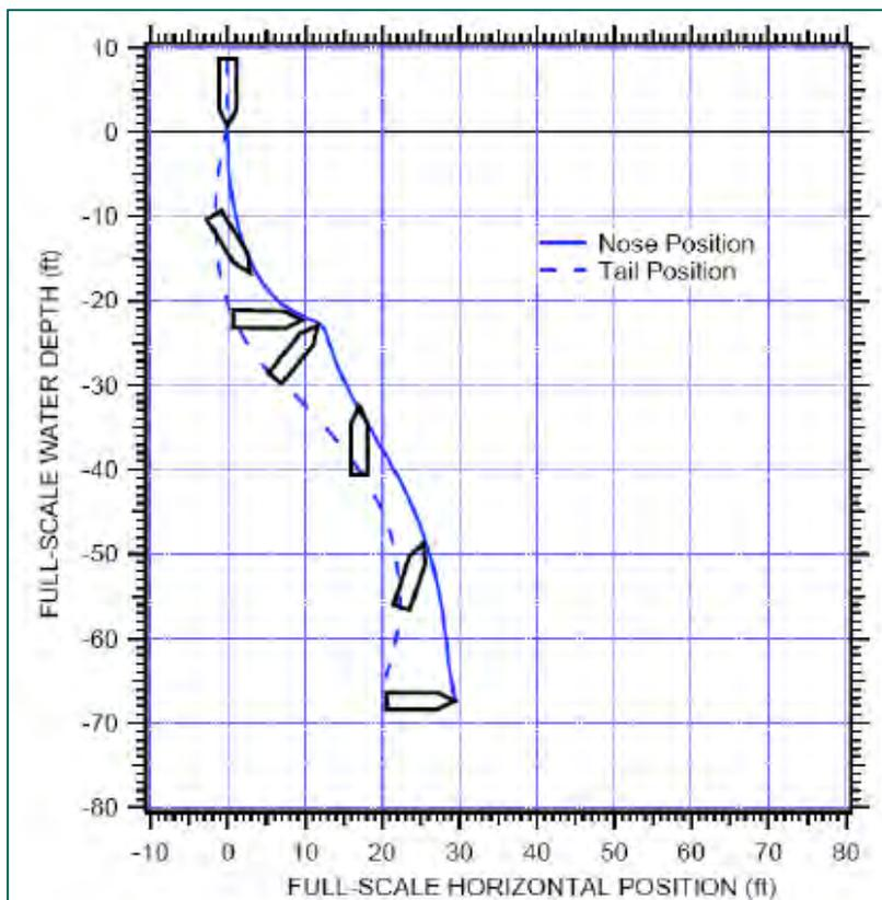
Figure 15: Trajectory of Mk 84 with no tail section and water-entry velocity of 296 m/s.
