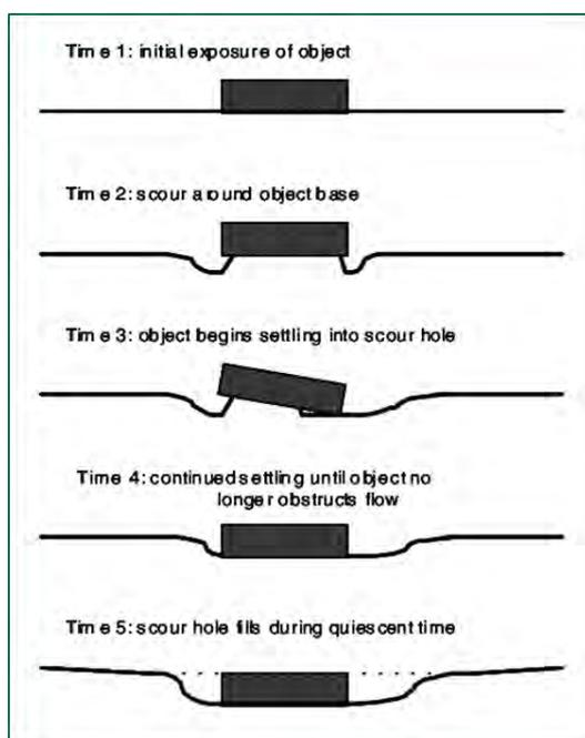
Figure 16: Scour mechanism<sup>10</sup>.
