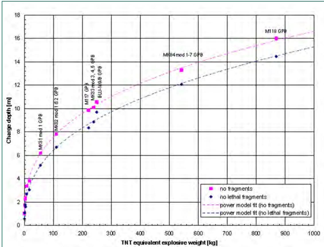
Figure 18: Minimal water depth to detain fragmentation of explosives with a Net Explosive Weight of 0-1,000 kg TNT equivalent [12].
