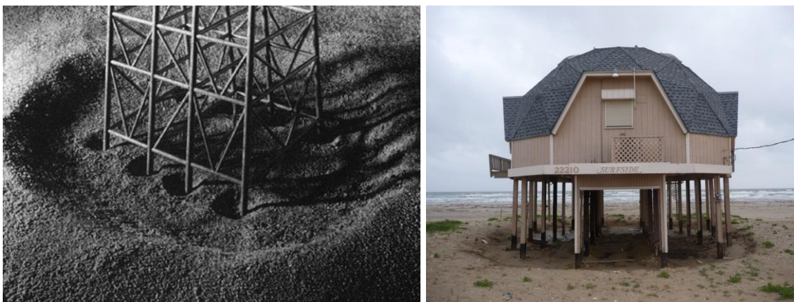
Figure 4.2 (Left) local scour holes around individual jacket legs and global scour pit around entire footprint observed in a scale model test [after Whitehouse, 1998]; (right) local scour holes around foundation piles and global scour hole around entire beach house after occurrence of Hurricane Ike.
