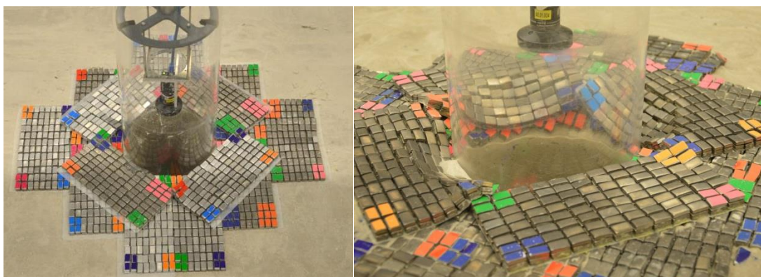
Figure 5.9 Example of a physical model test result of block mattresses around a monopile foundation before a test (left) and after. The small gaps between the mattresses close to the pile has led to some scour development.
