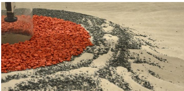
Figure 5.4 Falling apron of the filter layer, covering the slopes around the protection after a lowering of the surrounding seabed.
