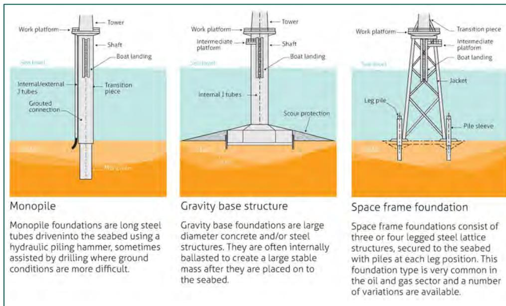
Figure 30: Example of suitable foundation types<sup>25</sup>.
