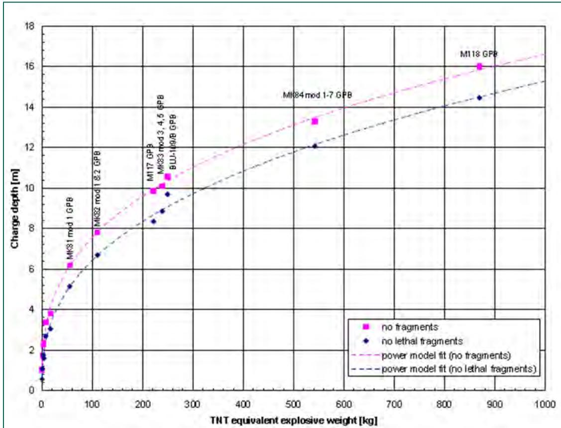
Figure 29: Minimal water depth to detain fragmentation of explosives with a Net Explosive Weight of 0-1,000 kg TNT equivalent [12].
