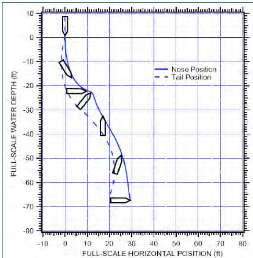
Figure 25: Trajectory of Mk84 with no tail section and water-entry velocity of 296 m/s.
