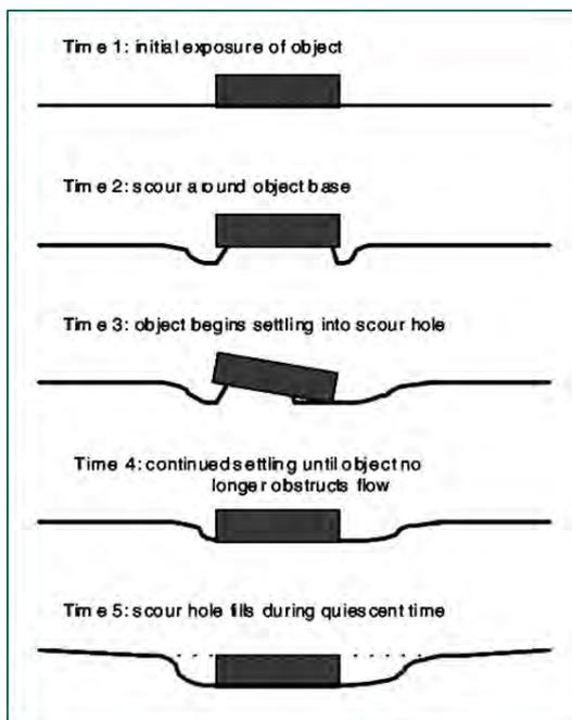
Figure 26: Scour mechanism<sup>8</sup>.
