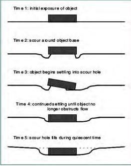
Figure 26: Scour mechanism<sup>8</sup>.
