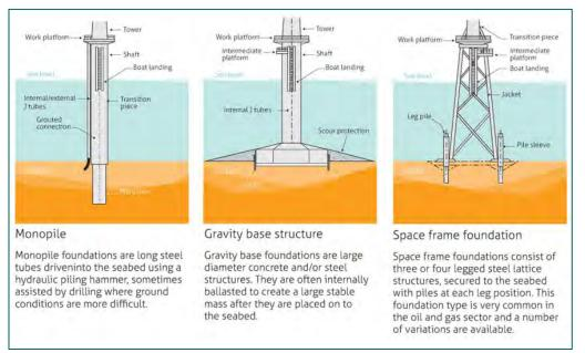
Figure 30: Example of suitable foundation types<sup>25</sup>.
