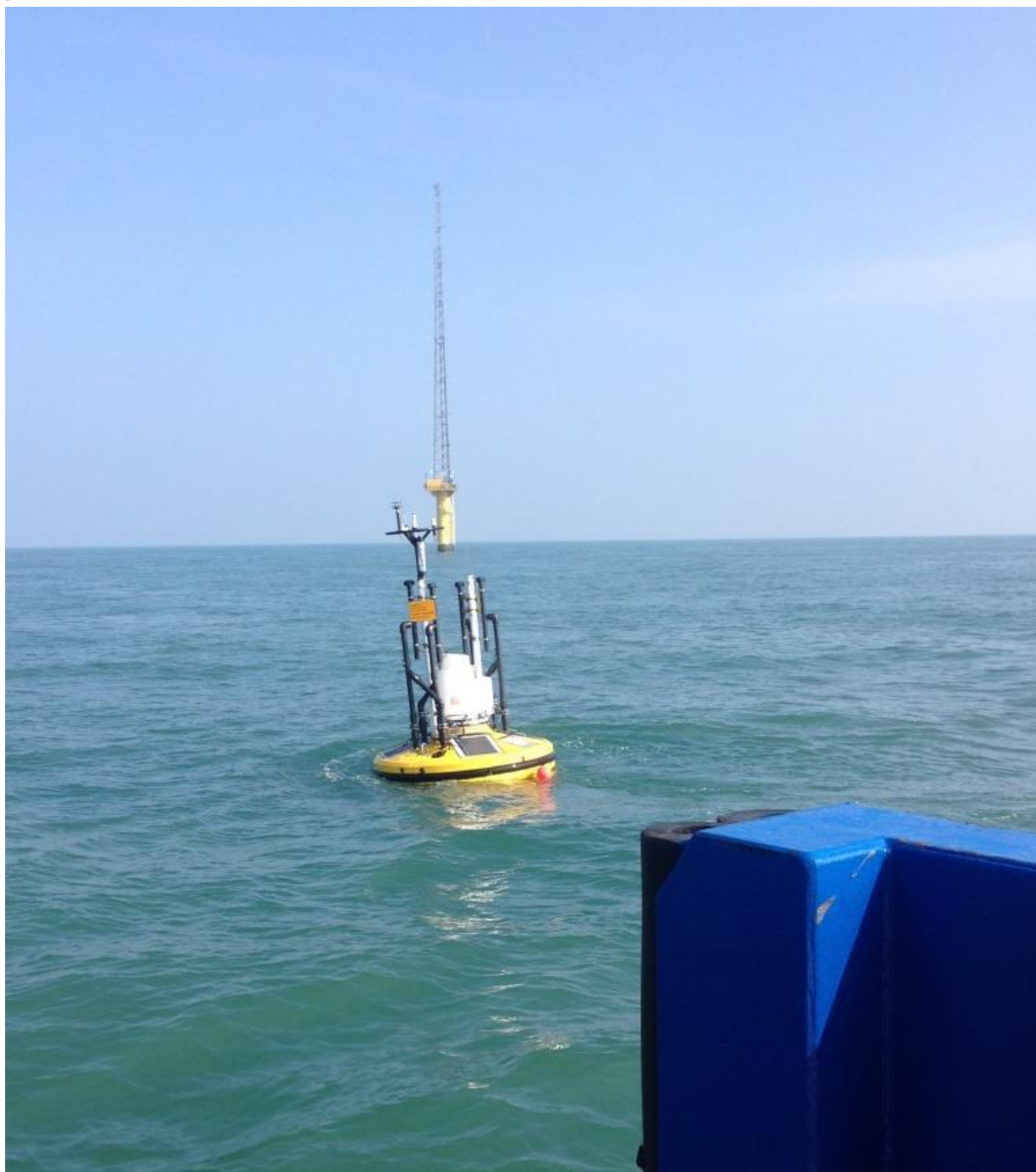
Figure A.2: SEAWATCH Wind LiDAR Buoy and EA1B mast
