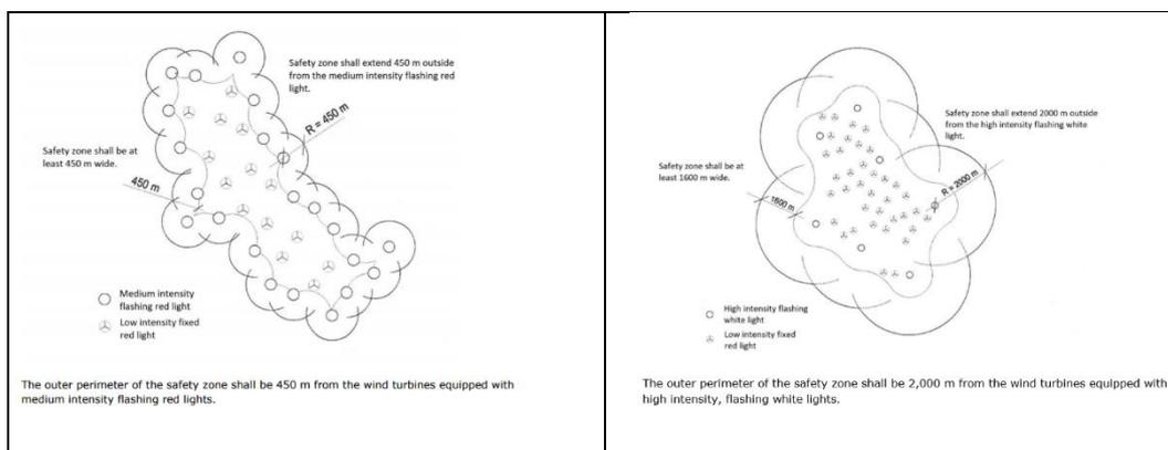
**Figure 8: Model of contour lighting from Finnish Transport Safety Agency**
