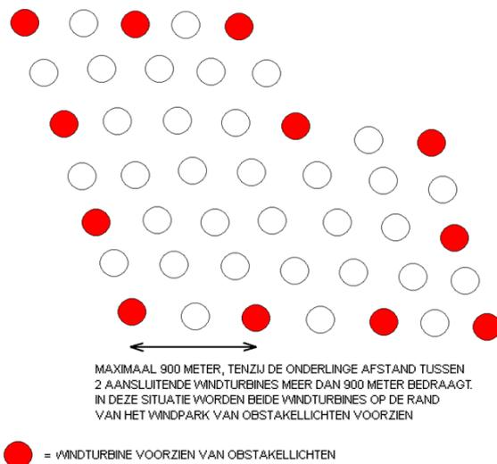
**Figure 7: Configuration contour lighting according to ILT *Informatieblad***
