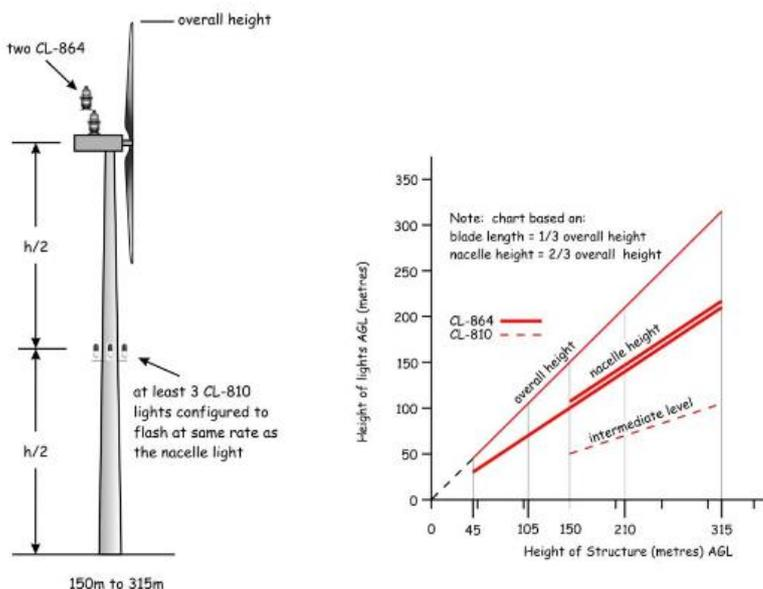
**Figure 3: Lighting wind turbines, heights 150m to 315m (source Canadian Standard 621)**
