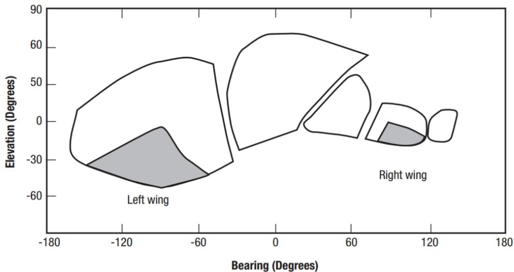
**Figure F-1 ATSB report showing field of sight limitations for a general aviation aeroplane**
