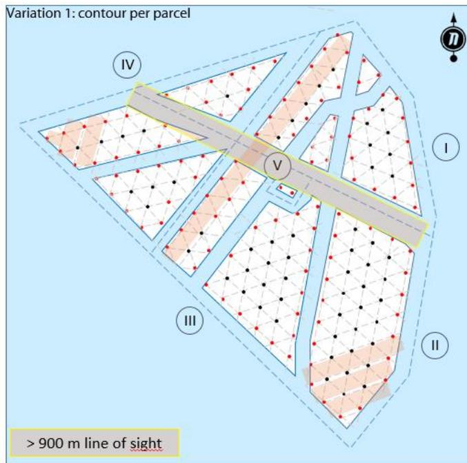
**Figure 11: Variation 1: Indicative layout of 1,200 Meter grid with contour lighting per parcel**
