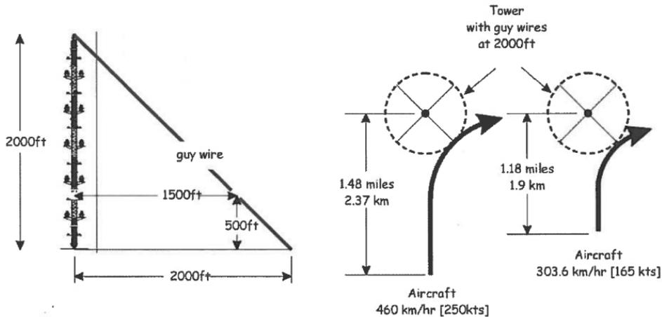
**Figure D-1 Visual distance communication tower**
