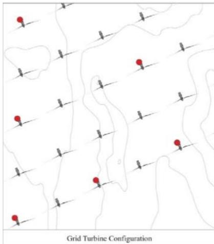
**Figure 9: Configuration grid lighting according to FAA Advisory Circular (AC) 70/7460-1L**
