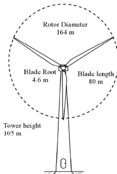
**Figure 2: Dimensions of a Vestas V164 wind turbine**
