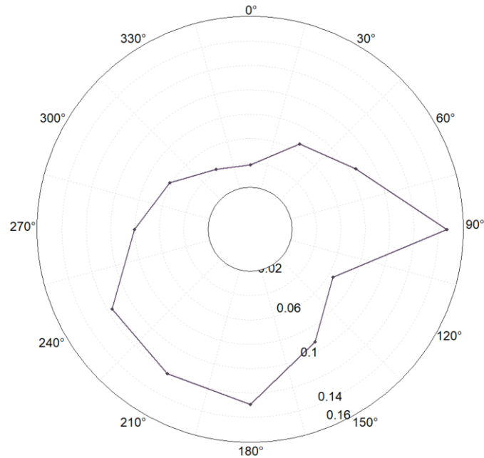
Figure 5-3. Modelled long-term wind shear rose at N4 (200 m, 140 m, 100 m wind speed)
