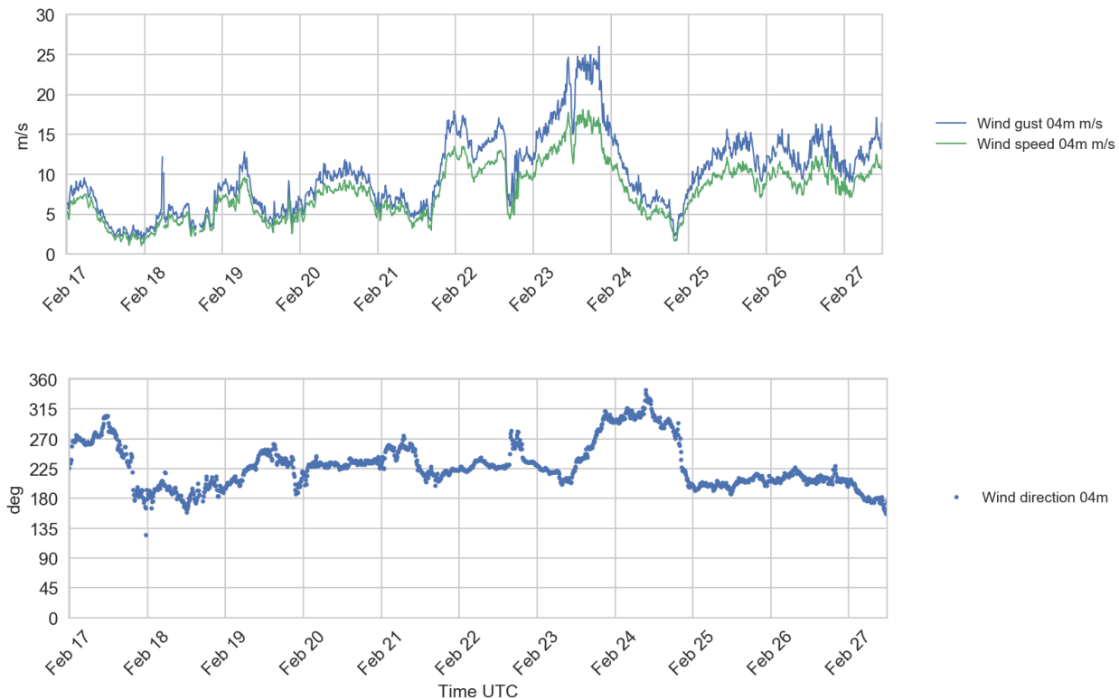
Figure 4.9 Plots of wind speed and gust (upper), and wind direction (lower) at 4 m a.s.l., 16 - 27 Feb 2017.
