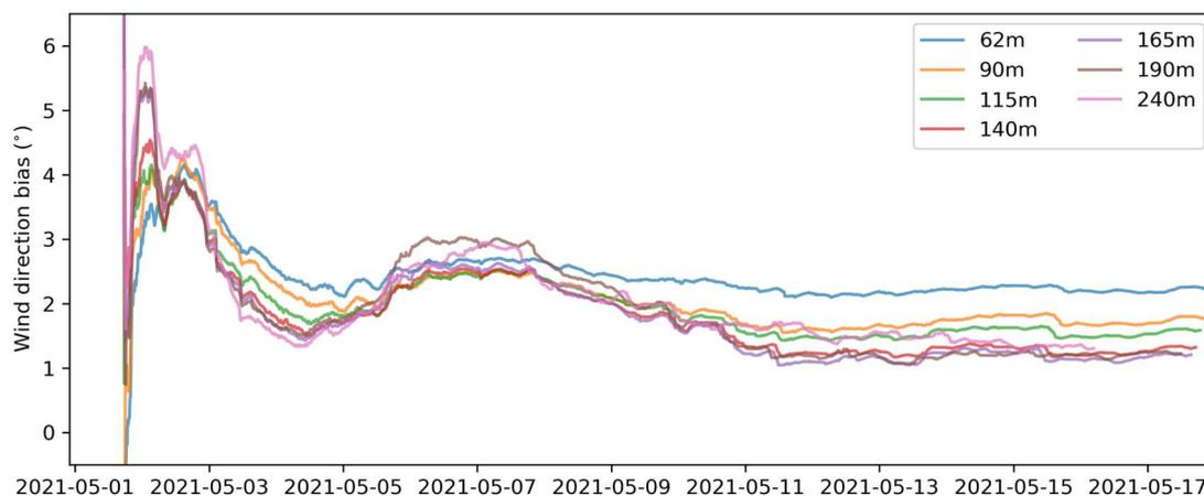
Figure 4-14: Temporal evolution of WS170 wind direction biases (mean wind direction difference) per height level after filtering for wind speeds > 2 m/s + banding. Number of samples used to calculate the biases increases in time.
