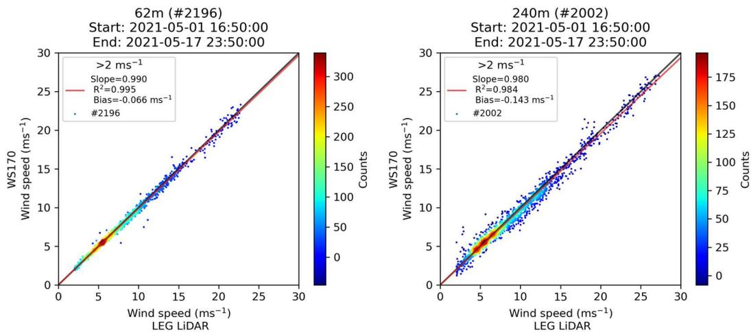
**Figure 4-11: Scatter plots comparing wind speeds > 2 m/s from LEG LiDAR and WS170 at 62m (left) and 240m (right).**
