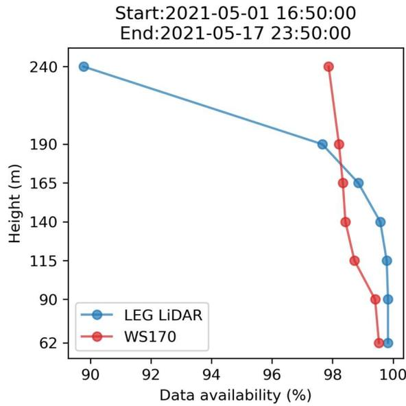
**Figure 4-6: Wind speed data availability for LEG LiDAR and WS170 during verification period.**
