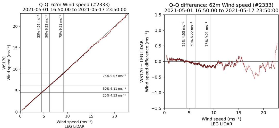
Figure 4-8: Quantile-Quantile (Q-Q) plot comparing quantiles of wind speeds measured at 62m by LEG LiDAR with WS170. Right: Difference between quantiles observed by WS170 and LEG LiDAR as a function of LEG LiDAR quantiles.
