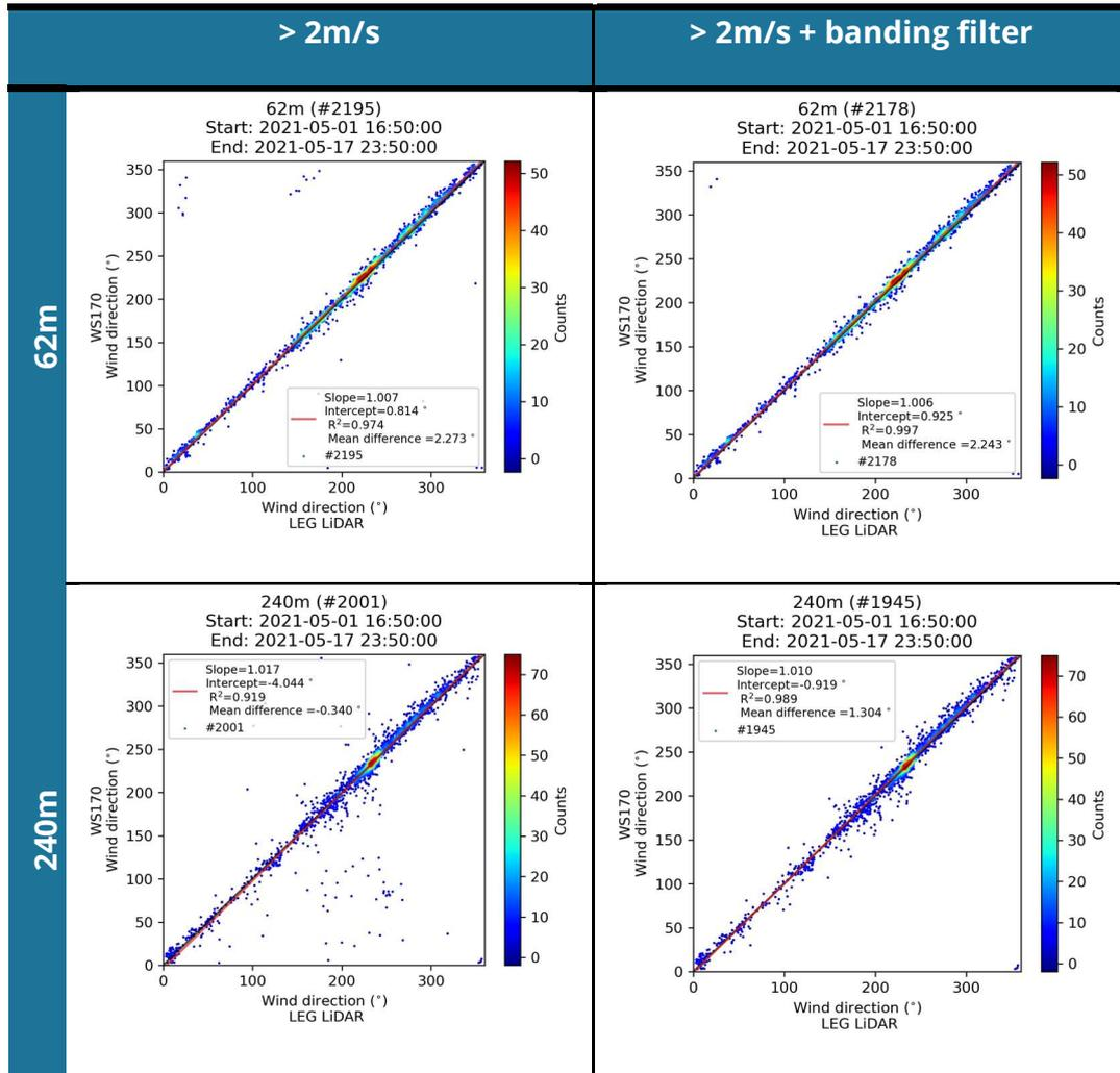
Figure 4-13: Scatter plots comparing wind directions from LEG LiDAR and WS170 at 62m and 240m for wind speeds > 2m/s and > 2m/s + banding filter.
