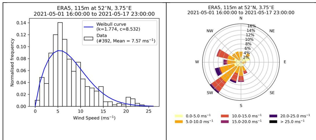
**Figure 4-1: Wind speed frequency histogram (left) and wind rose (right) derived from ERA5 hourly wind speeds (115m extrapolated from 100m using shear exponent between 10m and 100m) and wind directions (100m).**
