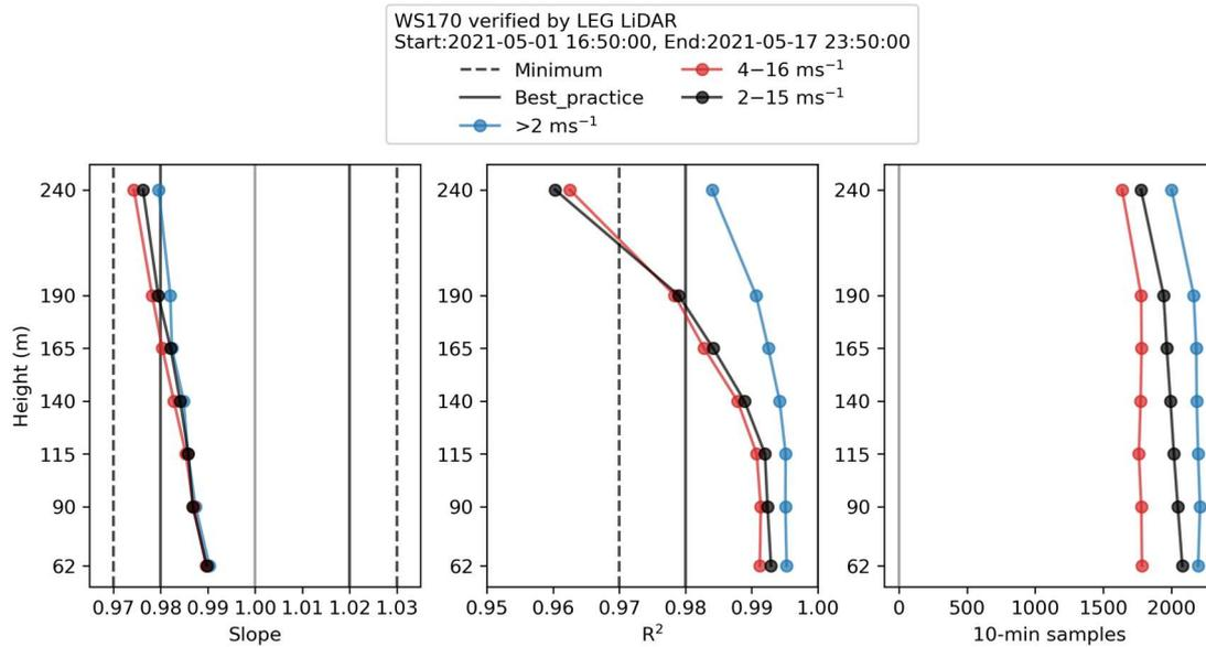
Figure 4-10: Slope, R<sup>2</sup> and number of samples for each wind speed verification test.
