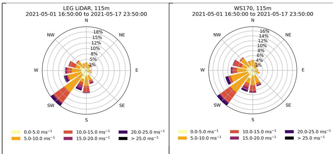
**Figure 4-3: Wind roses derived from 10-min wind speed and direction measurements at 115m from LEG LiDAR (left) and WS170 (right).**
