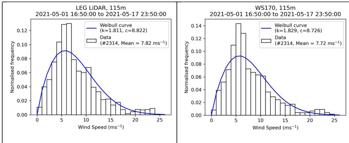
**Figure 4-2: 10-min wind speed frequency histograms and Weibull parameters at 115m from LEG LiDAR (left) and WS170 (right).**
