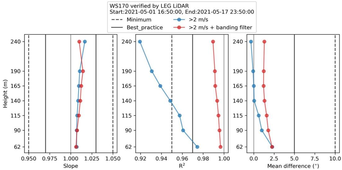
Figure 4-12: Slope,  $R^2$  and mean difference (bias) for wind direction verification tests.
