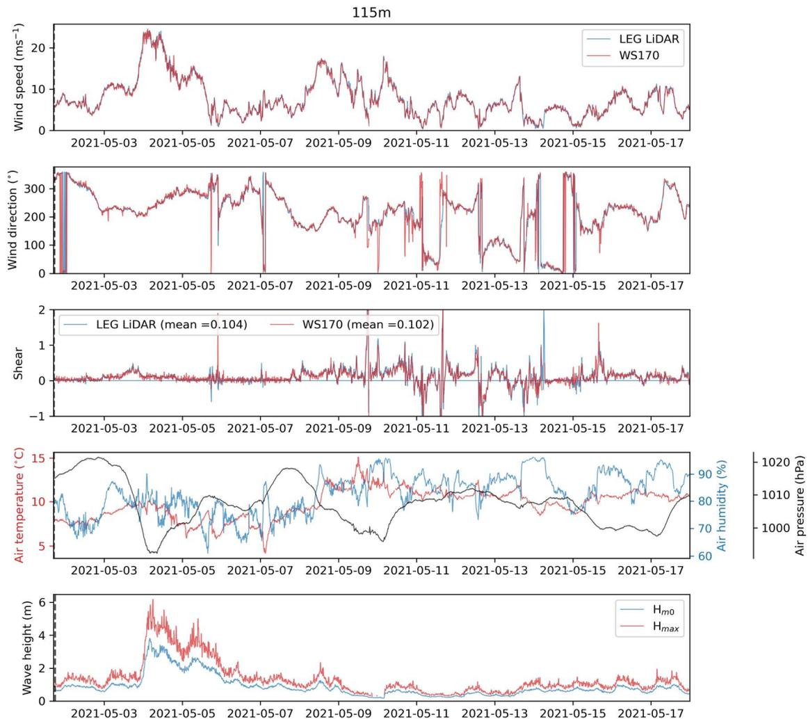
**Figure 4-4: Timeseries of 10-min measurements of 115m wind speed, 115m wind direction, vertical wind shear (shear exponent calculated between 62m and 115m wind speed) from LEG LiDAR and WS170; and air temperature, humidity, air pressure and wave height at WS170.**
