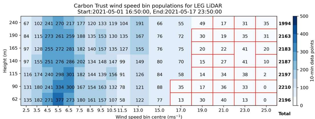
**Figure 4-7: Binned wind speed data populations per height level from LEG LiDAR measurements during verification period. Data are binned according to the Carbon Trust protocol. Red boxes**
