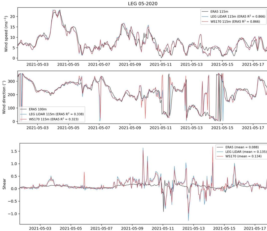
**Figure 4-5: Timeseries of hourly 115m wind speed, wind direction and vertical wind shear (power law exponent) estimated by ERA5, LEG and WS170. The shear exponent is calculated using 10m and 100m wind speeds in ERA5 and 62m and 115m wind speeds in LEG and WS170.**
