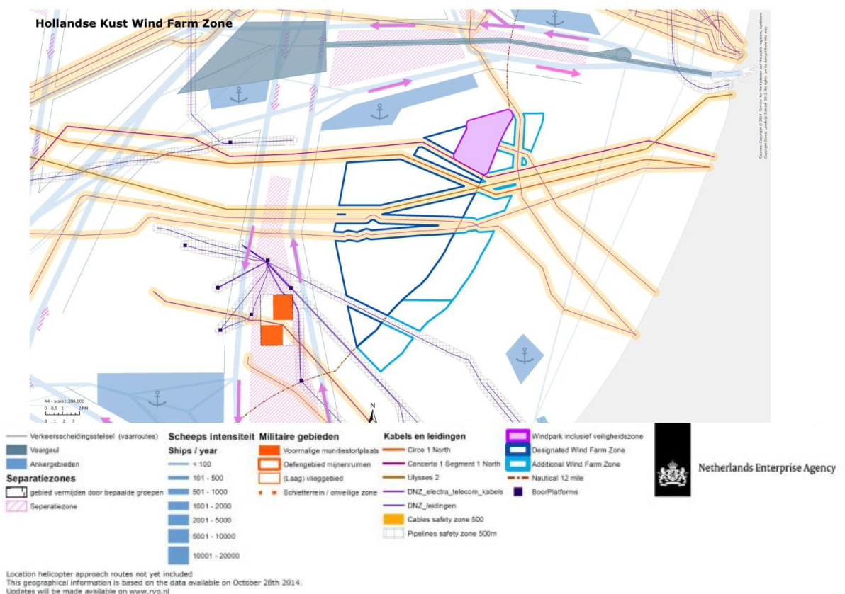
Figure 3.2 Overview of (sub-)site division in the HKZWFZ (blue lines), its intended additional zone (light blue lines) and safety zones related to telecommunication and electricity cables (crossing the area from west to east).
