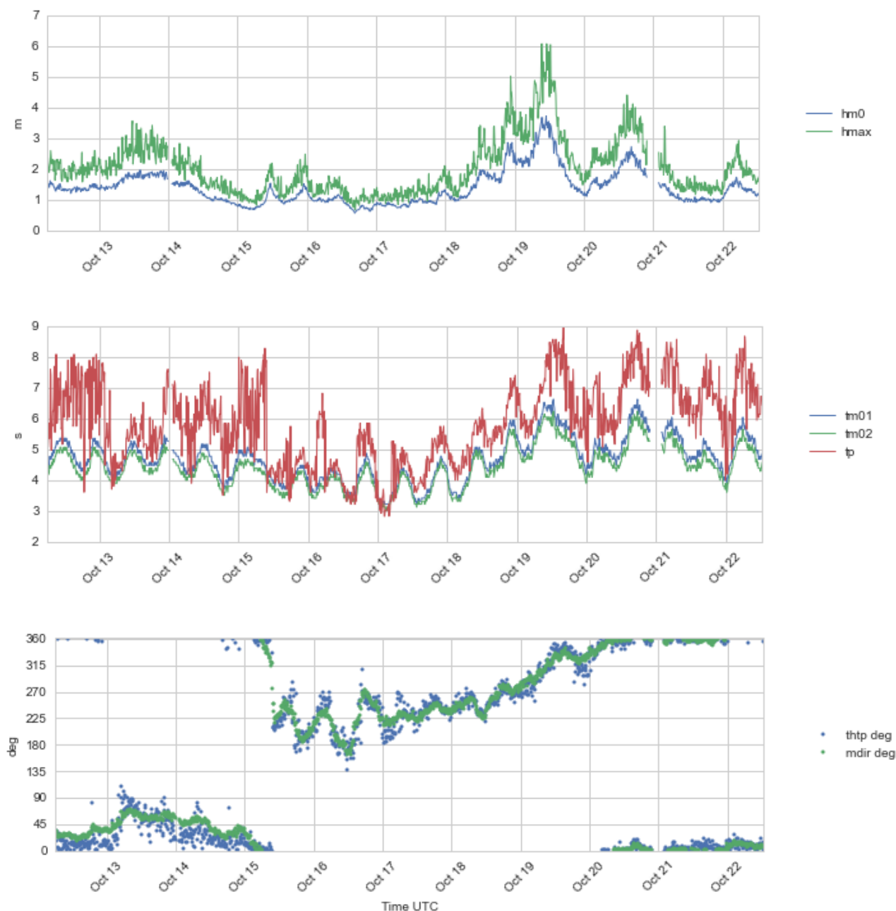
Figure 4.6 Time series plots of wave height ( H_{m0} and H_{max} ) (upper panel), wave period ( T_{m01} , T_{m02} and T_p ) (second panel), and wave direction ( ThTp and Mdir ) (lower panel), 12 - 22 Oct 2016.
