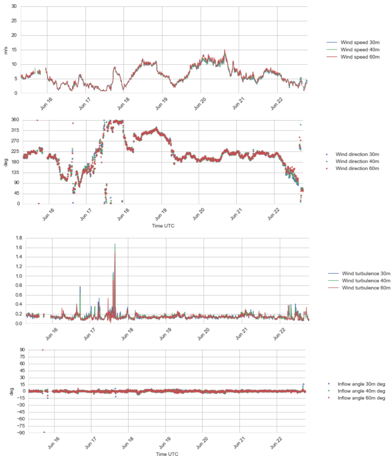
Figure 4.7 Plots of wind profile data, 30 – 60 m a.s.l., 15 - 22 Jun 2016.
