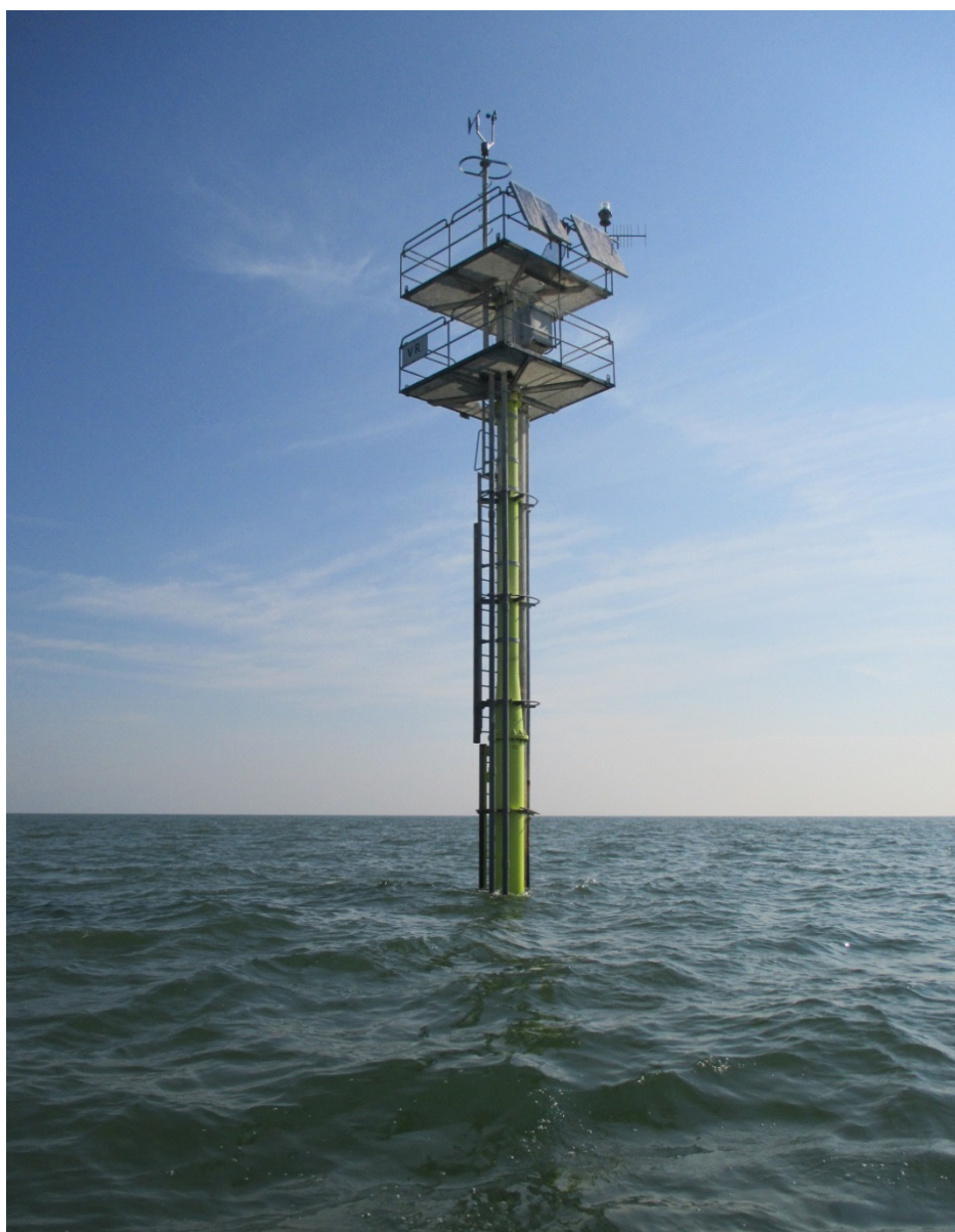
Figure 3.2 The wind measuring station at Vlakte van de Raan.
