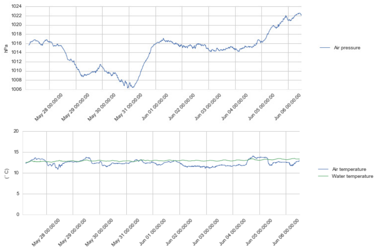
Figure 4.2 Time series plots of air pressure (upper panel), air and water temperature (lower panel), 27 May – 6 Jun 2016.
