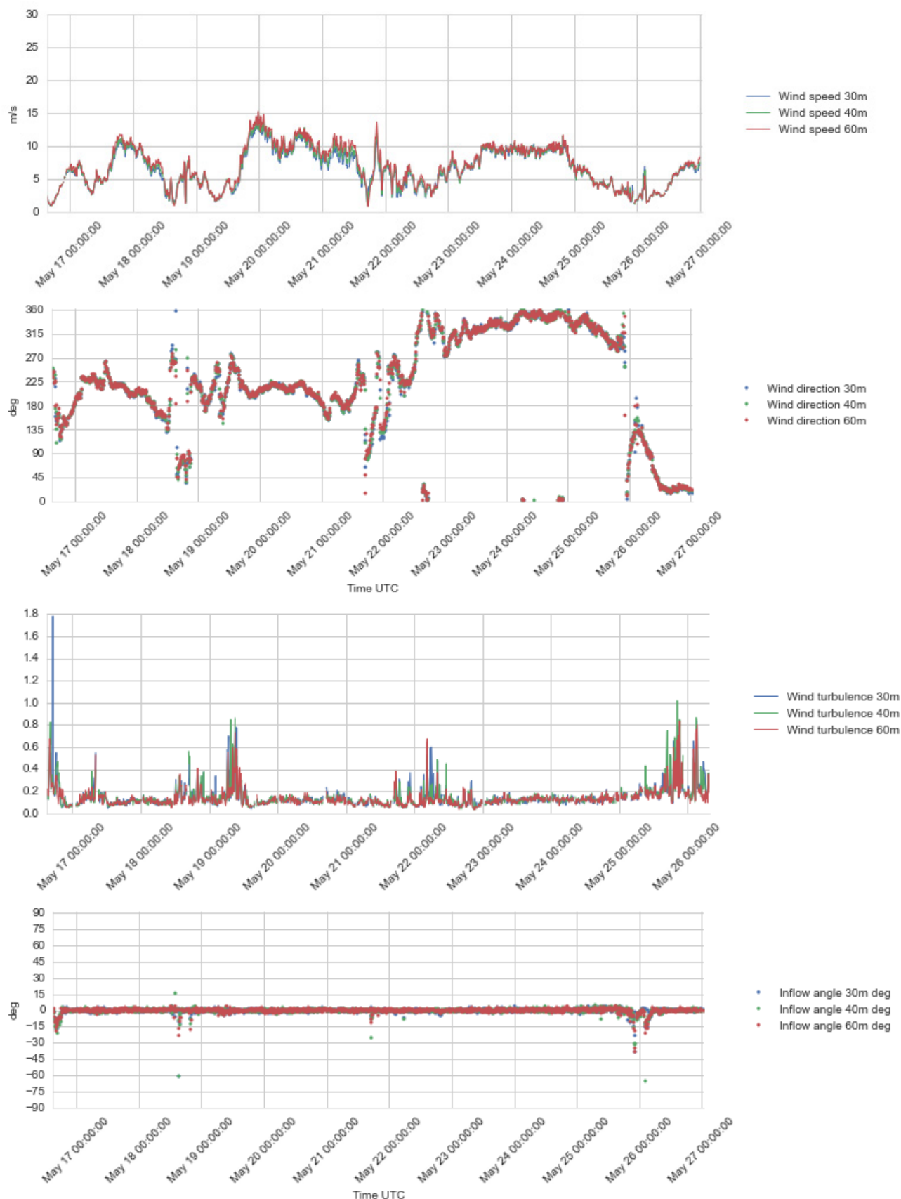
Figure 4.10 Plots of wind profile data, 30 – 60 m a.s.l., 16 – 26 May 2016.
