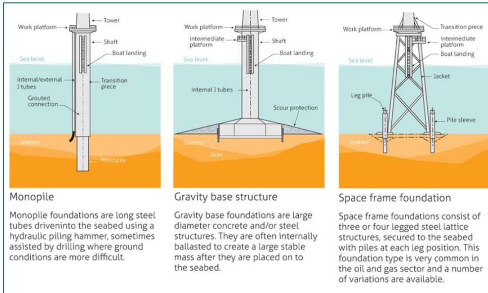
Figure 24: Example of suitable foundation types [21].
