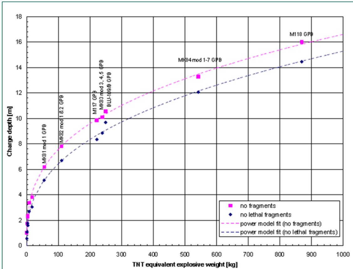
Figure 23: Minimal water depth to detain fragmentation of explosives with a Net Explosive Weight of 0-1,000 kg TNT equivalent [12].
