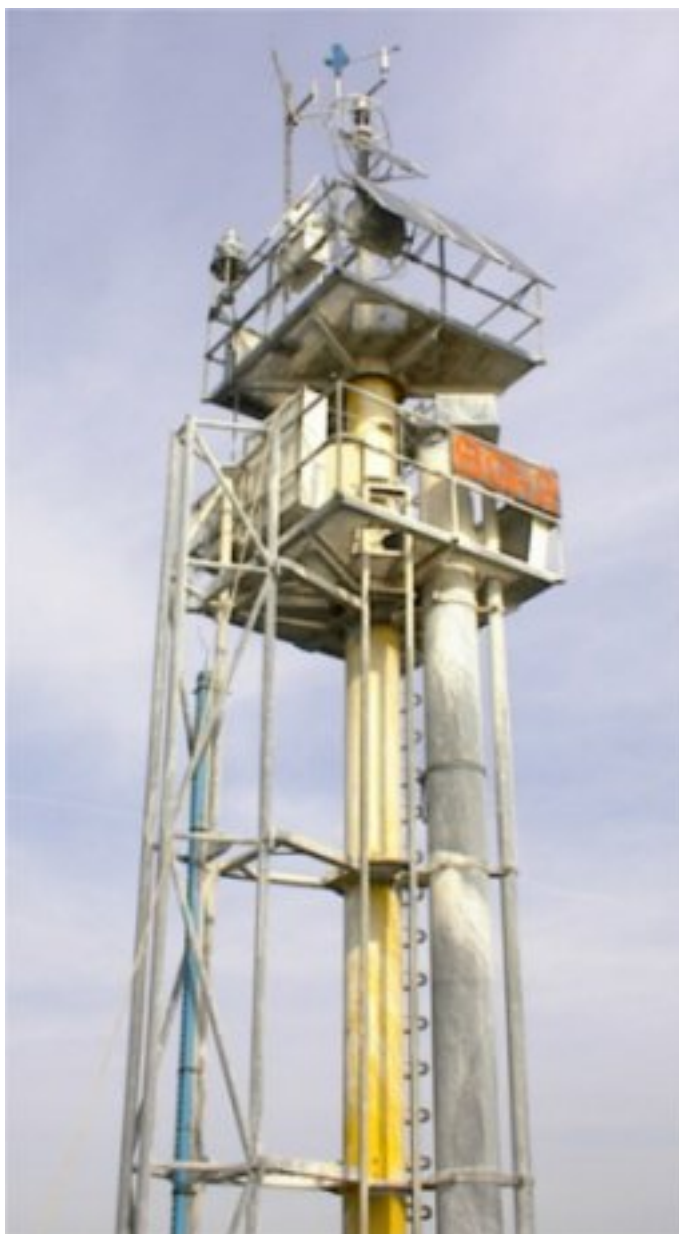
Figure 3.3 The meteorological mast station at Brouwershavensegat (BG2) showing the locations of the wind sensors on the top deck.
