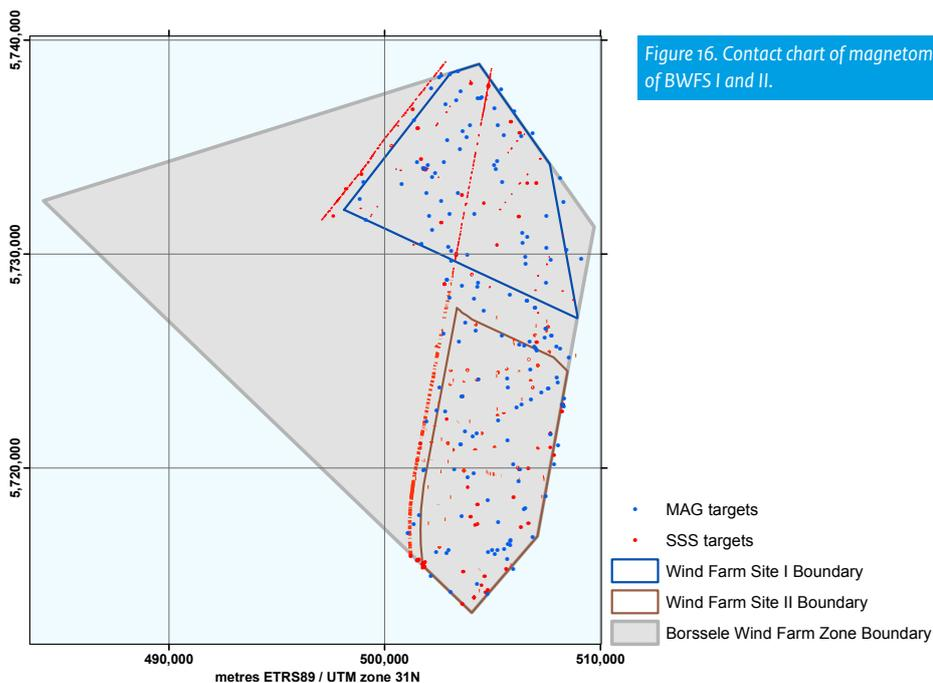
Figure 16. Contact chart of magnetometer and side-scan sonar survey of BWFS I and II.
