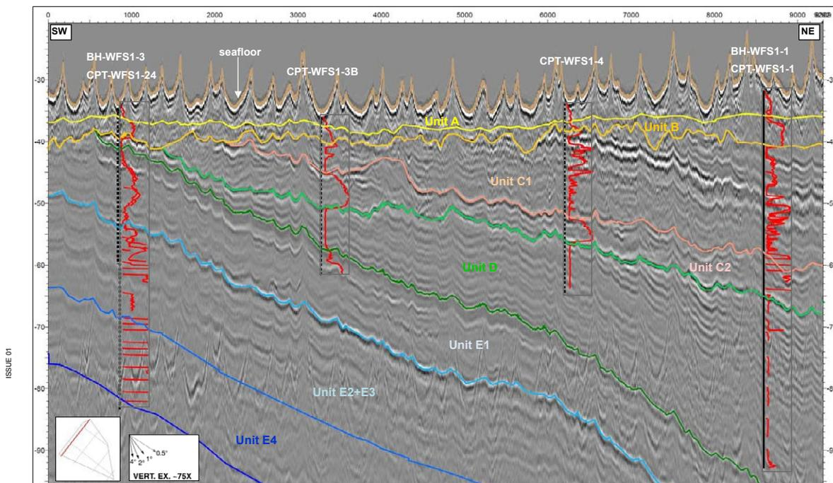
NOTE: Example of MCS seismic line (vertical and horizontal scales are in metres).
