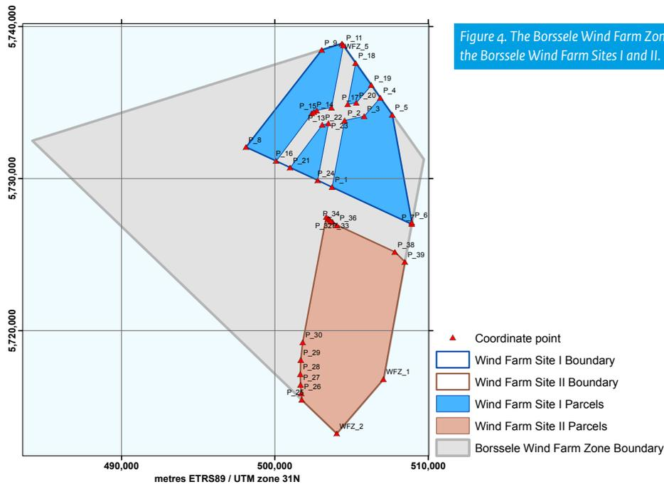
Figure 4. The Borssele Wind Farm Zone and the corner coordinates of the Borssele Wind Farm Sites I and II.
