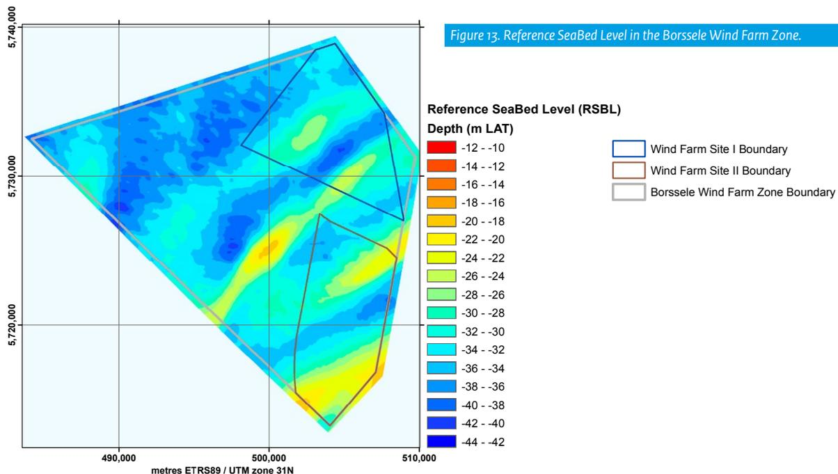
Figure 13. Reference SeaBed Level in the Borssele Wind Farm Zone.
