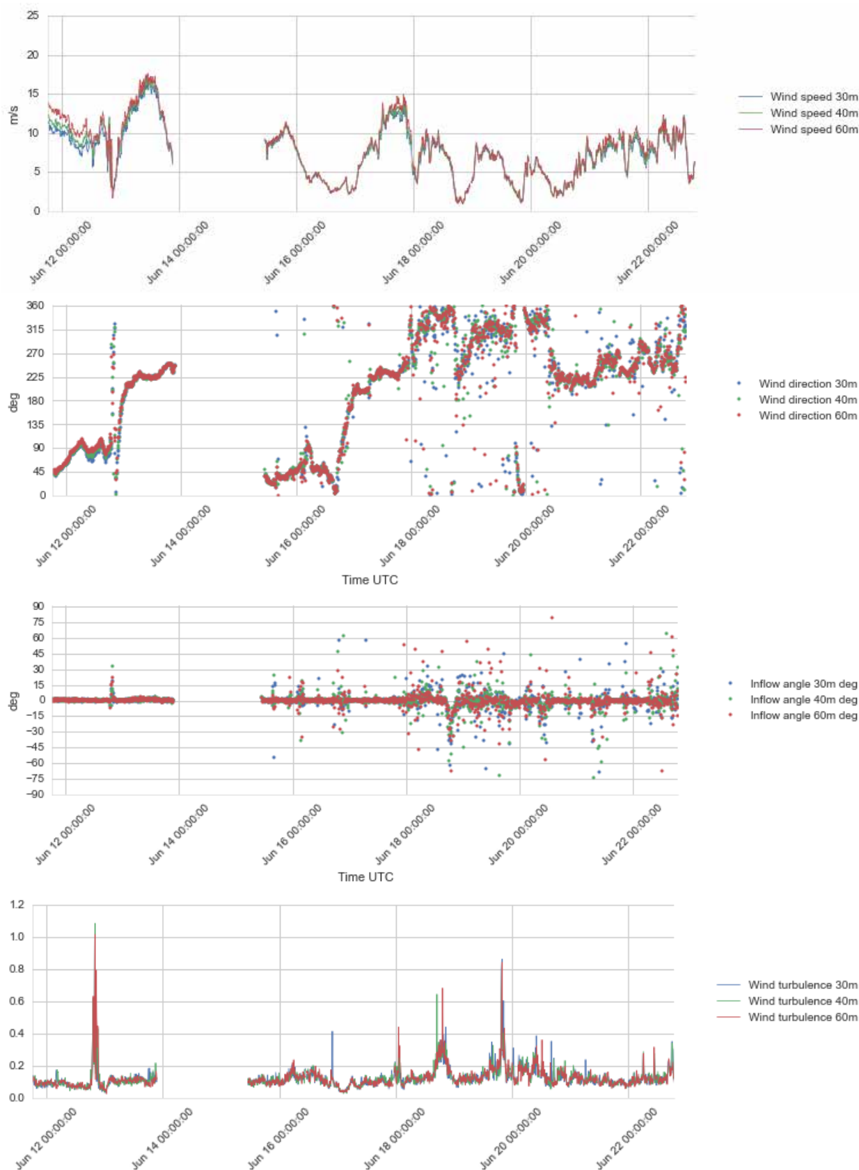
Figure 4.10 Plots of wind profile data, 30 – 60 m a.s.l., 11 - 22 June 2015.
