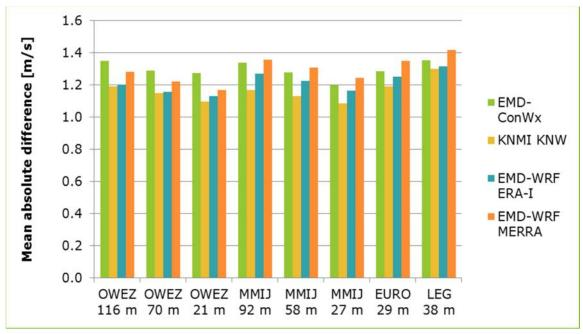
Figure 39 – Mean absolute difference in wind speed between mesoscale and measured datasets
