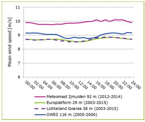
Figure 20 – Mean diurnal profile of wind speed for four measurement locations. The top measurement heights show very little diurnal variation, as is typical offshore.
