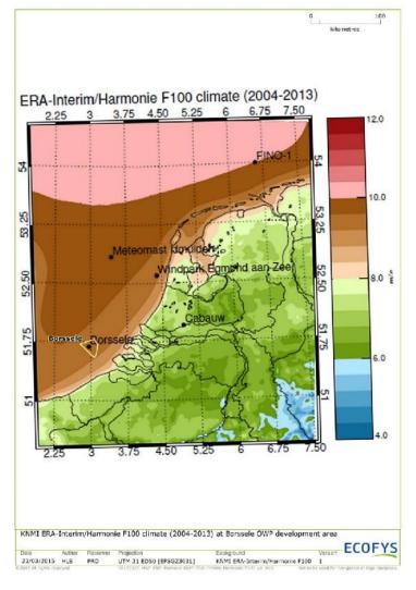
Figure 13 - Borssele zone and the KNMI NoordzeeWind (KNW) offshore wind atlas
