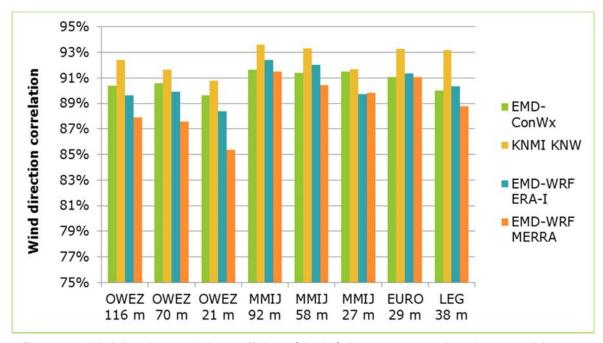
Figure 37 – Wind direction correlation coefficients (circular), between mesoscale and measured datasets
