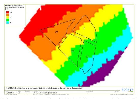
Figure 12 – Long-term corrected mean wind speed at 100 m for the Borssele zone, as calculated by the EU project NORSEWInD, Focus Area 2
