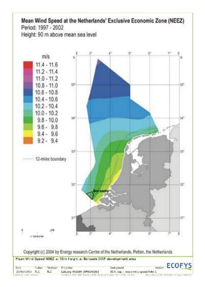
Figure 10 - Borssele zone and the ECN offshore wind atlas (2004 version)
