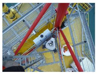
Figure 7 - LiDAR located within the lattice structure of the Meteomast IJmuiden offshore met mast [source: ECN]
