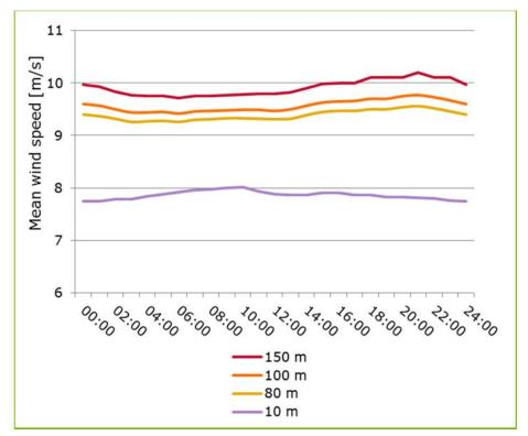
Figure 19 - Mean diurnal profile of wind speed, at the centre of the Borssele zone
