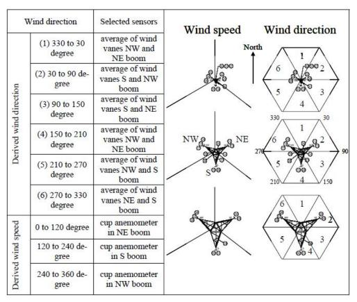
Figure 34 - Overview of ECN data processing rules for the OWEZ mast data to obtain derived wind speed and wind direction from undisturbed sensors only.
