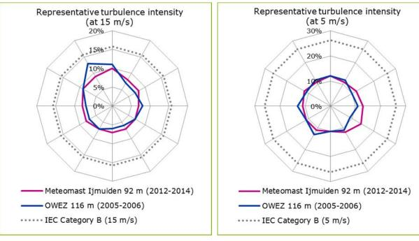
Figure 32 – Measured representative turbulence intensity at OWEZ and Meteomast IJmuiden, for wind speeds of 15 m/s (left) and 5 m/s (right). The IEC limits for Category B wind turbines are also shown.
