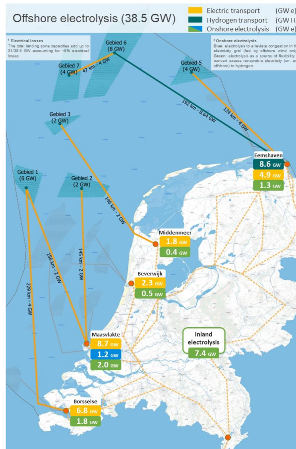
Figure 33: Configuration for solution involving offshore electrolysis.
