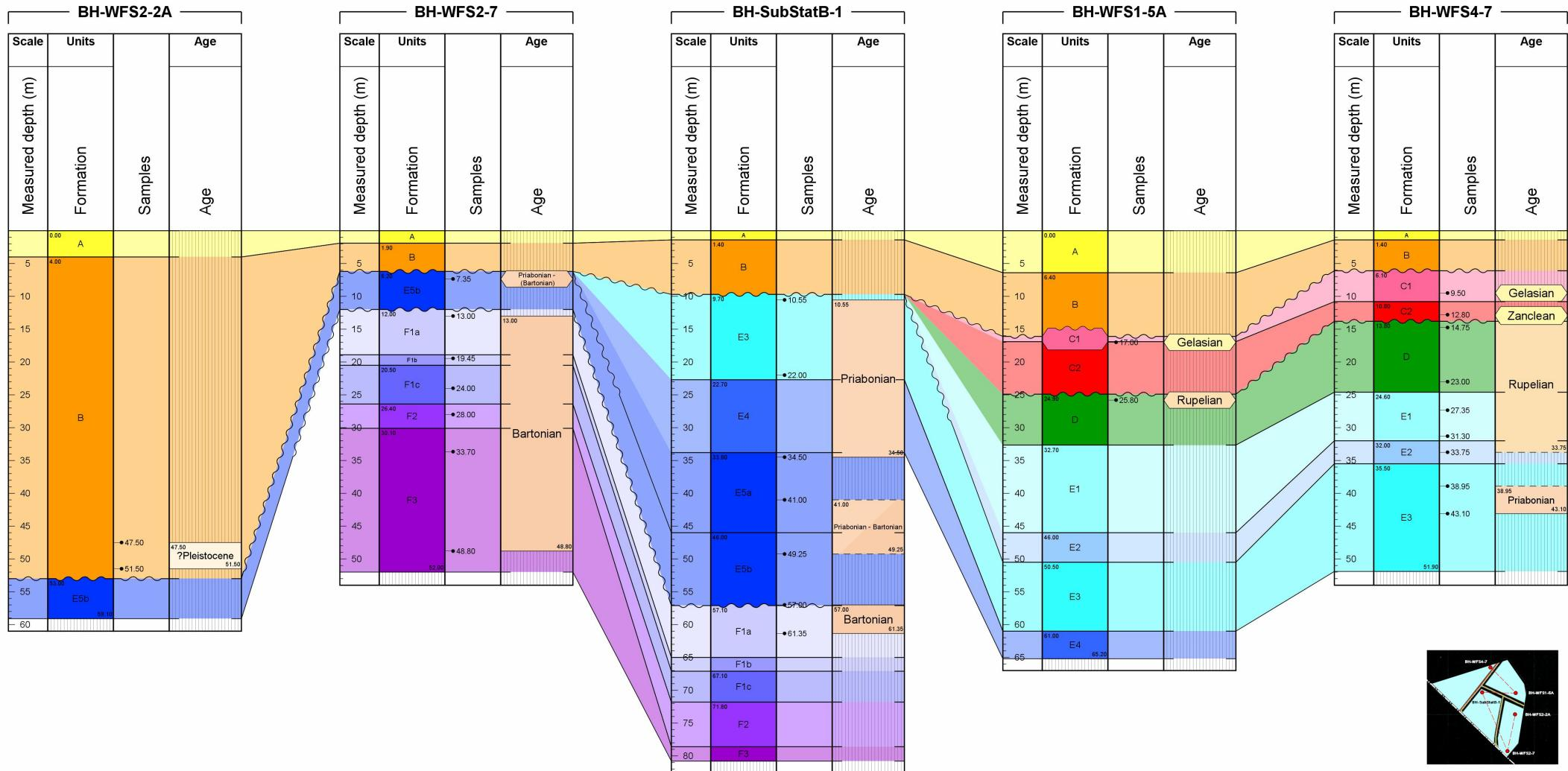
Correlation of studied boreholes based on proposed Geotechnical Units and showing biostratigraphic ages determined in the study.
