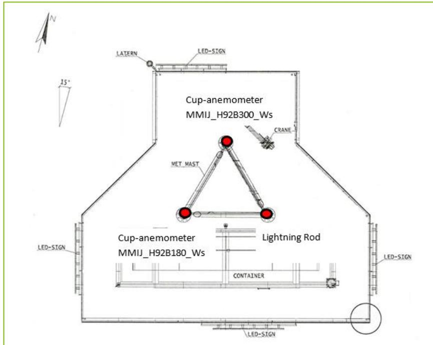
Figure 35 - Top view of 92 m top section of met mast IJmuiden (source: [6]) with the location of the two cup-anemometers and the lightning rod indicated.
