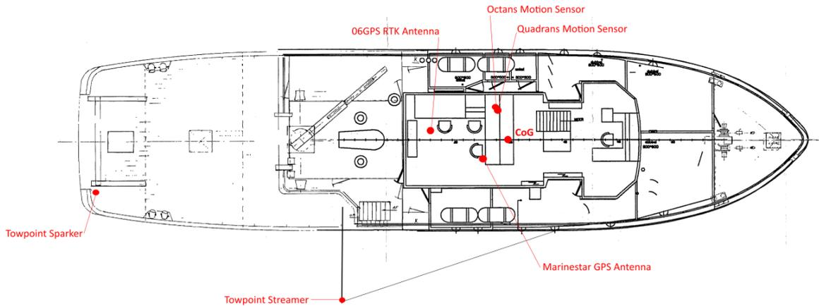
Figure 5-4: MV Seazip Surveyor vessel offset diagram
