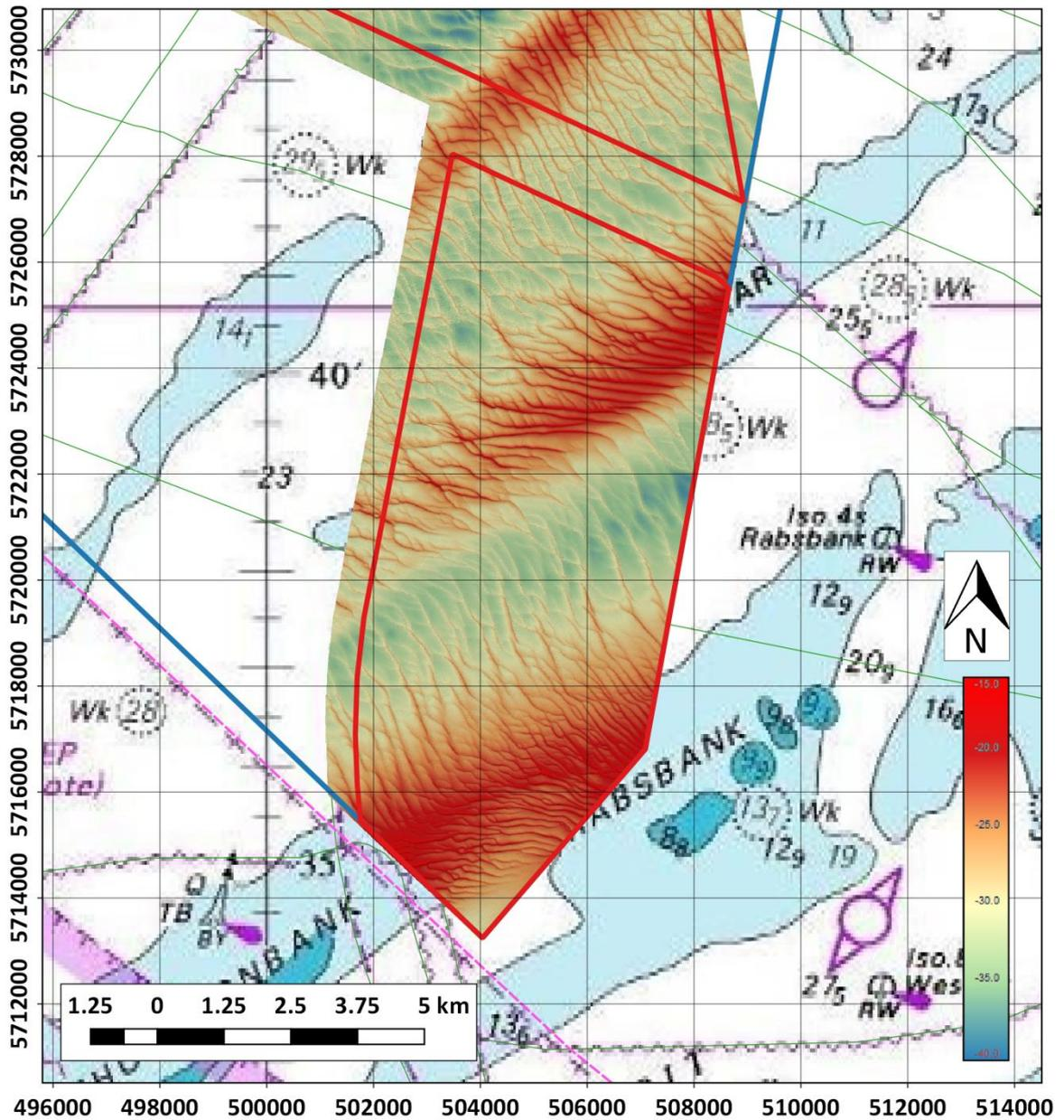
Figure 3-3: WFS-2 MBE survey grid superimposed on the nautical chart
