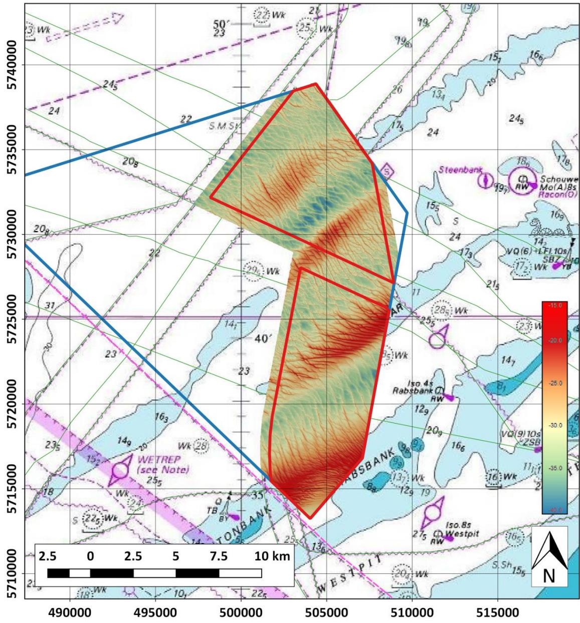
Figure 3-2: WFS-1 and WFS-2 MBE survey grid superimposed on the nautical chart
