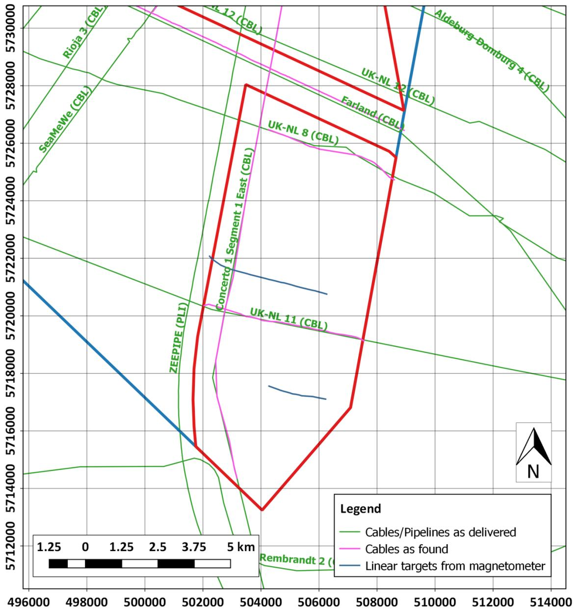
Figure 3-8: Overview map of cables and pipelines in WFS-2, as found and as provided by the client
