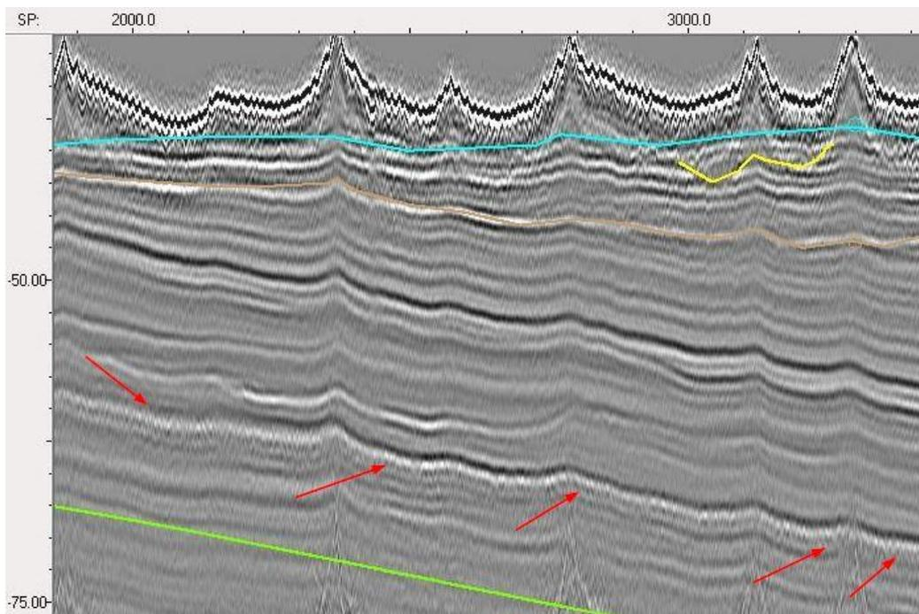
Figure 3-42: Evidence of gravel and boulders in U4.
